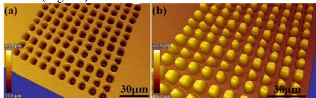
Fig. 1. Images of (a) ablated master, and (b) PDMS-mould.
