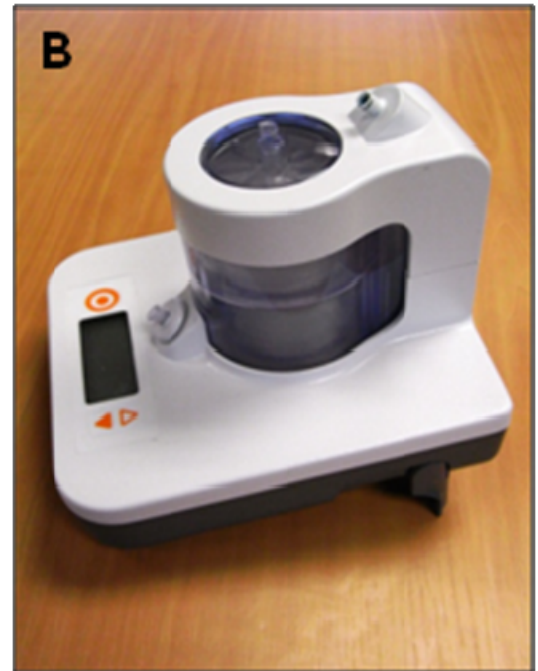
Figure 1A-B: Product concept of vacuum-assisted acoustic-filtration device, designed for single use within the sterile operating field. C: Prototype laboratory device used in this study for analysis of BMA from a cohort of elderly patients.
