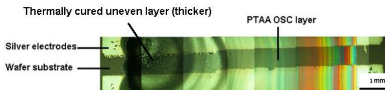
Figure 105. One inkjet printed transistor on a silicon dioxide coated silicon wafer with channel length of 1 mm.
