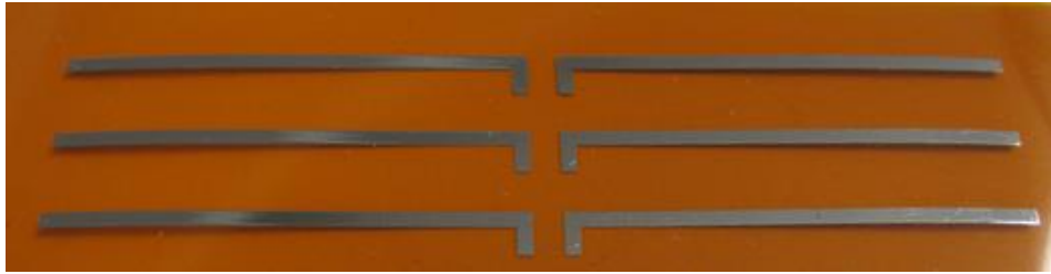
Figure 32. Plan view of three inkjet printed 2.4 GHz dipole antennas on Kapton.
