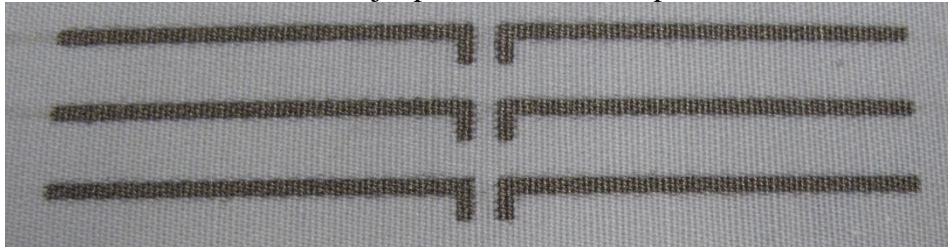
Figure 34 Plan view of three inkjet printed 2.4 GHz dipole antennas on standard fabric.
