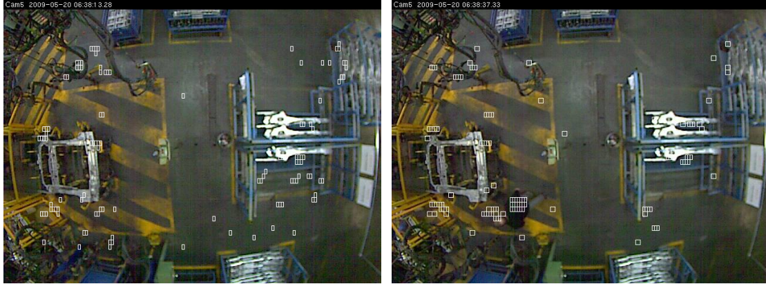
(a) Person free image: Randomly distributed spurious detections (b) Image with a Person: Multiple compact detections around the person in image
