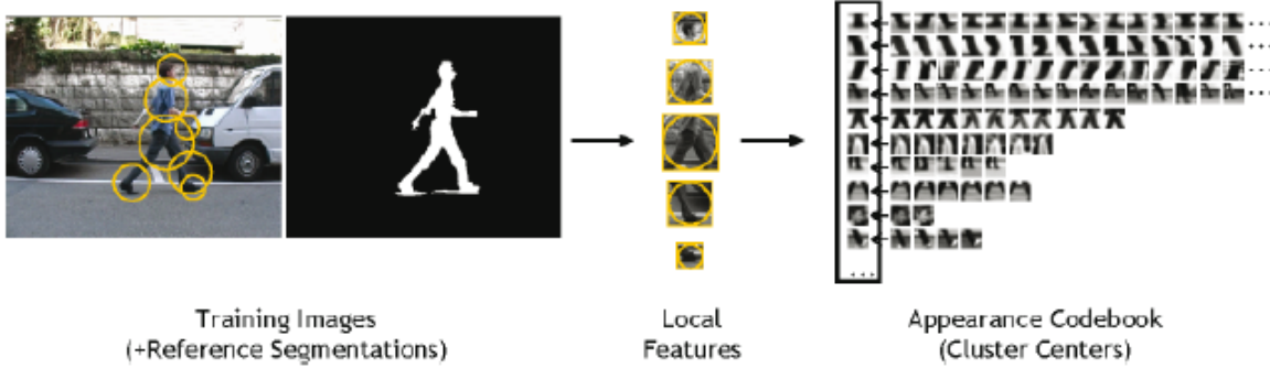
FIGURE 2.16: The training process of person detection system using the Implicit Shape Model (from [68]).
