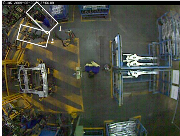
FIGURE 1.8: Context knowledge: Box 1 contains a person while box 2 is perceived as a human by the computer due to a lack of common sense knowledge.
