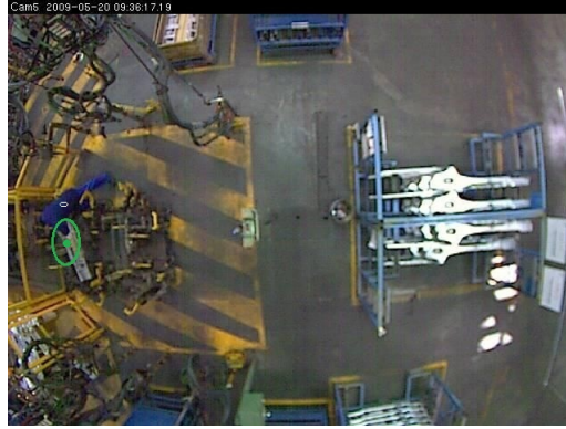
FIGURE 6.10: Test sequence 1. In this image, instead of a person, a steel rod is considered as a moving blob (shown in a green ellipse) by the Mean-Shift algorithm.
