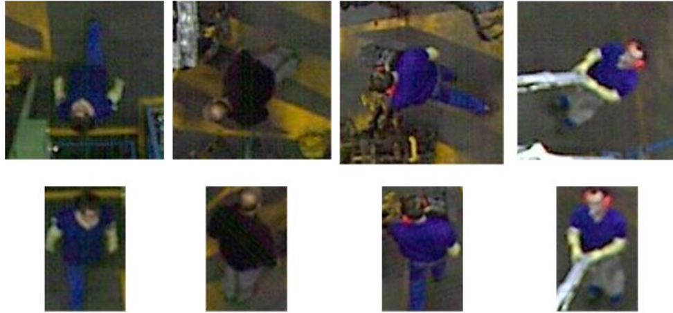
FIGURE 4.11: Orientation of people in images before applying rotation (row 1) and after applying rotation (row 2)
