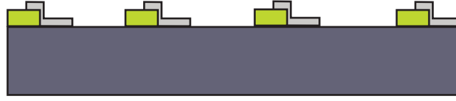
Figure 5.2: Illustration of the double metal strip-line LPD multiplex emitter
