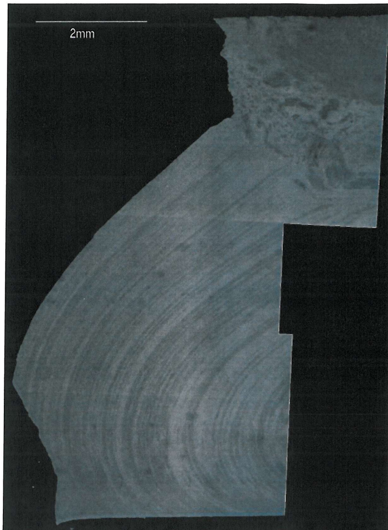
Figure 76 Macrograph showing the fatigue crack path down through the weld region.
