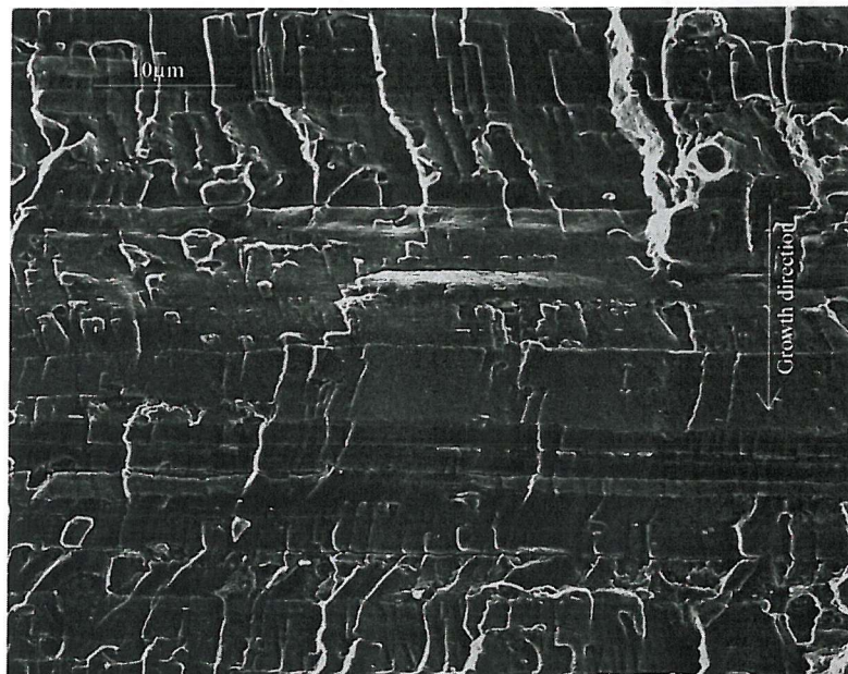
Figure 69 Higher \Delta K crack growth for failure outside the nugget region.
