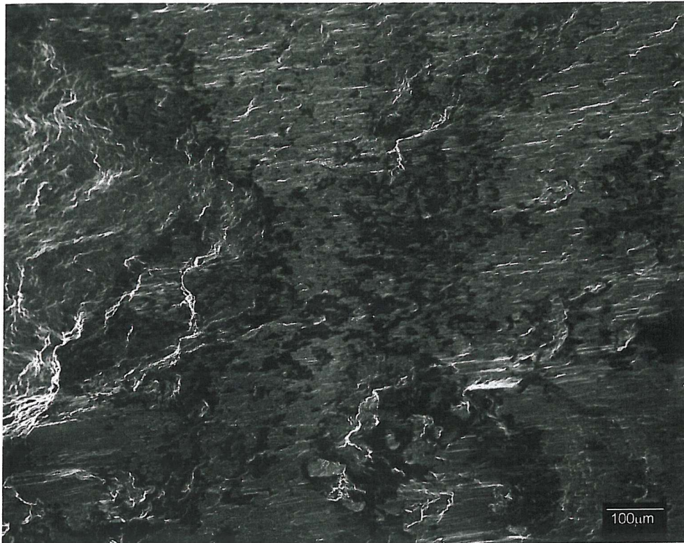
Figure 130 Fracture surface of subsurface crack deflection showing significant oxide debris and rubbing indicative of closure.
