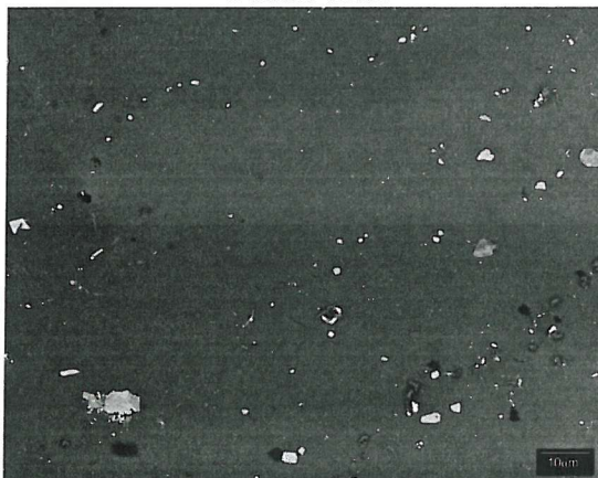
Figure 72 BEI Image of Macroscopic surface discontinuity, a) Low magnification with coarse and fine intermetallic sides labelled together with the interface, b) coarse intermetallic side and c) fine intermetallic side.
