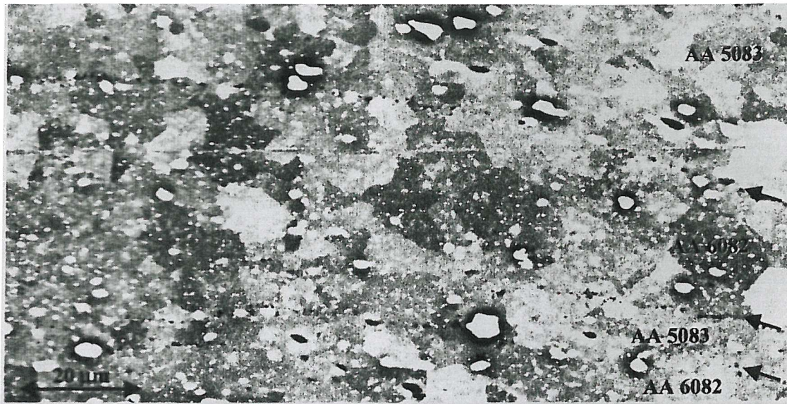
Figure 89 BEI image within the weld nugget in a dissimilar alloy friction stir weld of 5083 and 6082, highlighting dark oxide particles (arrows) delineating boundaries between 5083 and 6082 regions. 116
