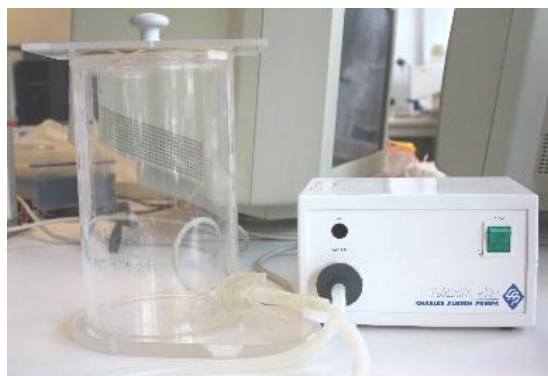
Figure III10. Formic eluent was degassed before daily analysis to avoid the formation of excessive bubbles by using this vacuum pump.
