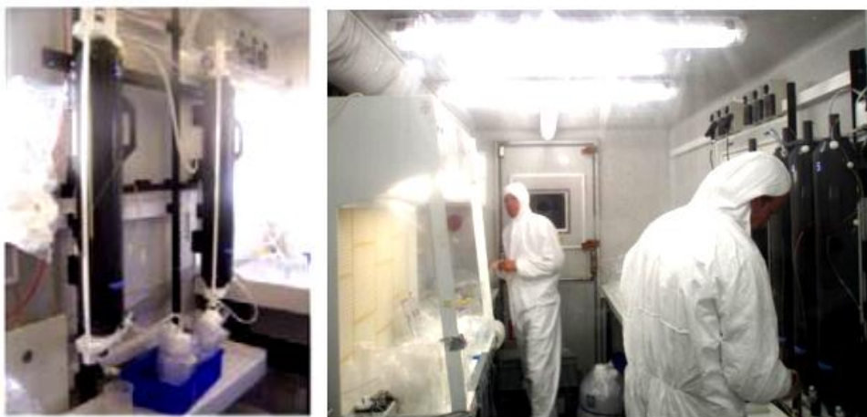
Figure II.2. Left: OTE bottles for the filtration of dissolved manganese. Right: trace metals sampling work in the clean container.
