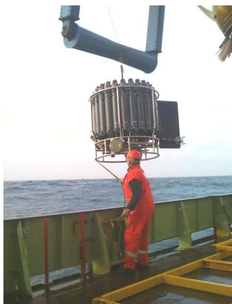
Figure II1. Example of Titanium-frame CTD rosette system as used to collect water column samples for trace metal work.
