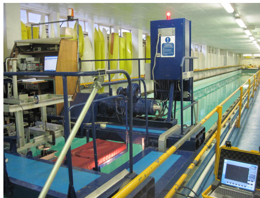
Figure 5.6: Southampton Solent Towing tank with carriage and acquisition equipment
