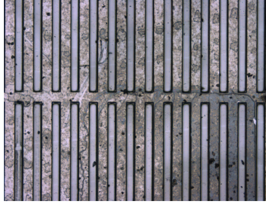
Figure 4.23: Microscope image of 100\mu m ridges using 5\times optical zoom
