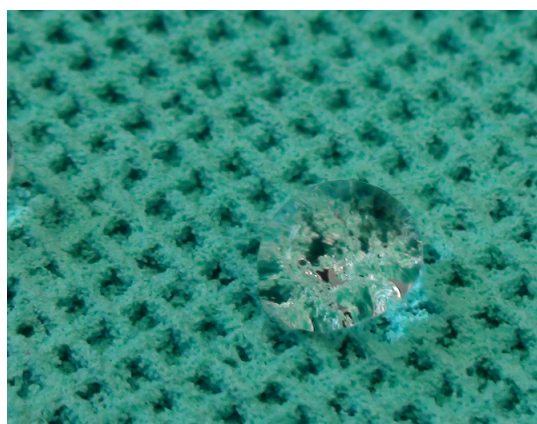
Figure 4.17: Coarse hydrophobic copper mesh with droplet and areas of high reflectivity showing the presence of a plastron
