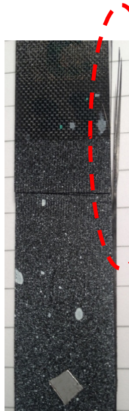
Figure 122: Longitudinal splitting of fatigued CFRP specimen at right specimen edge.
