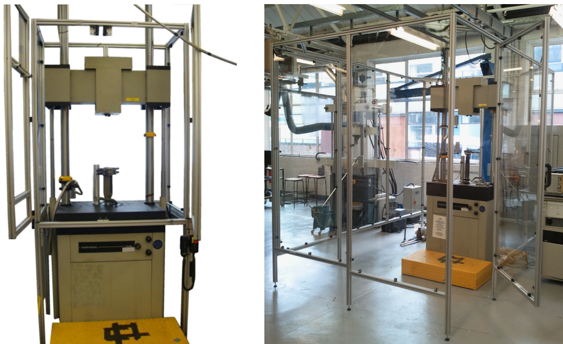
Figure 26: The Instron VHS 80/20 machine and the old (left) and new (right) protective enclosure.
