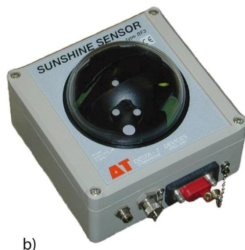
Figure 1.4.4 Diagram of direct PAR and b) the BF3 Sunshine Sensor that can be indirectly used to evaluate the direct PAR
