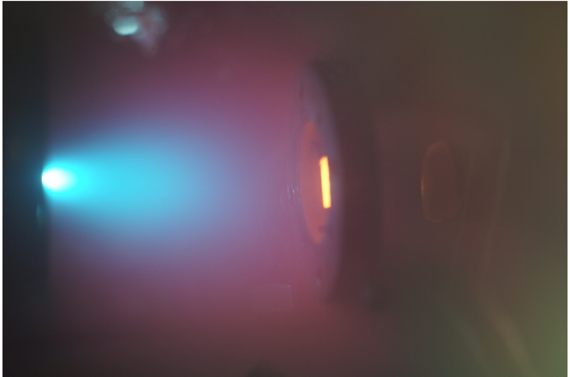
Figure 3.2.2. Plume formed by ablating a YIG target with a KrF laser at a fluence of F_{\text{KrF}} \approx 3 \text{ J/cm}^2 in \text{O}_2 .
