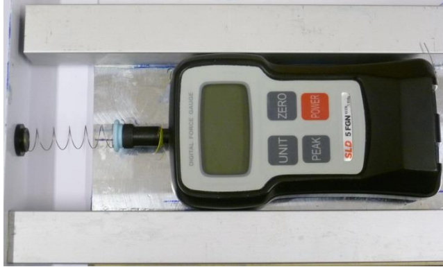
Figure 5.7 Measurement setup showing the two aluminium bars used to shape a channel to ensure the force meter moves along the central axis of the spring.
