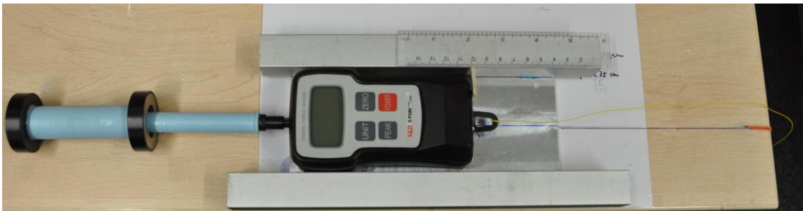
Figure 5.23 Photo of the measurement setup to evaluate the spring stiffness of the magnetic spring.
