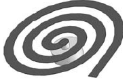
Figure 2.22 Schematic diagram of a spiral-shaped piezoelectric beam. (Reproduced from [83]).
