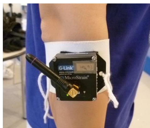
Figure 3.2 The accelerometer G-link mounted on the elbow using an elastic band.
