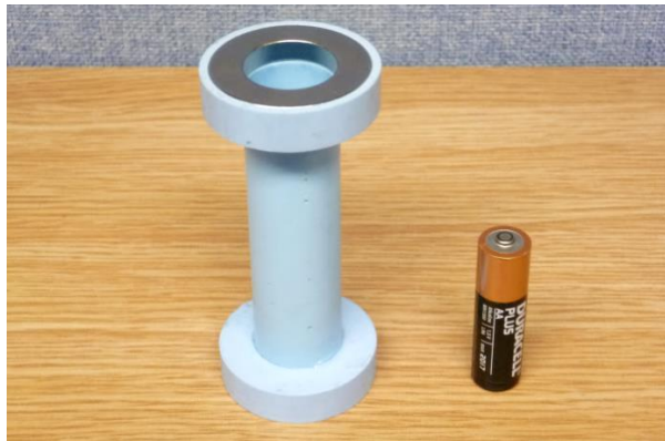
Figure 5.21 Photograph of the prototype of the magnetic spring alongside an AA battery.
