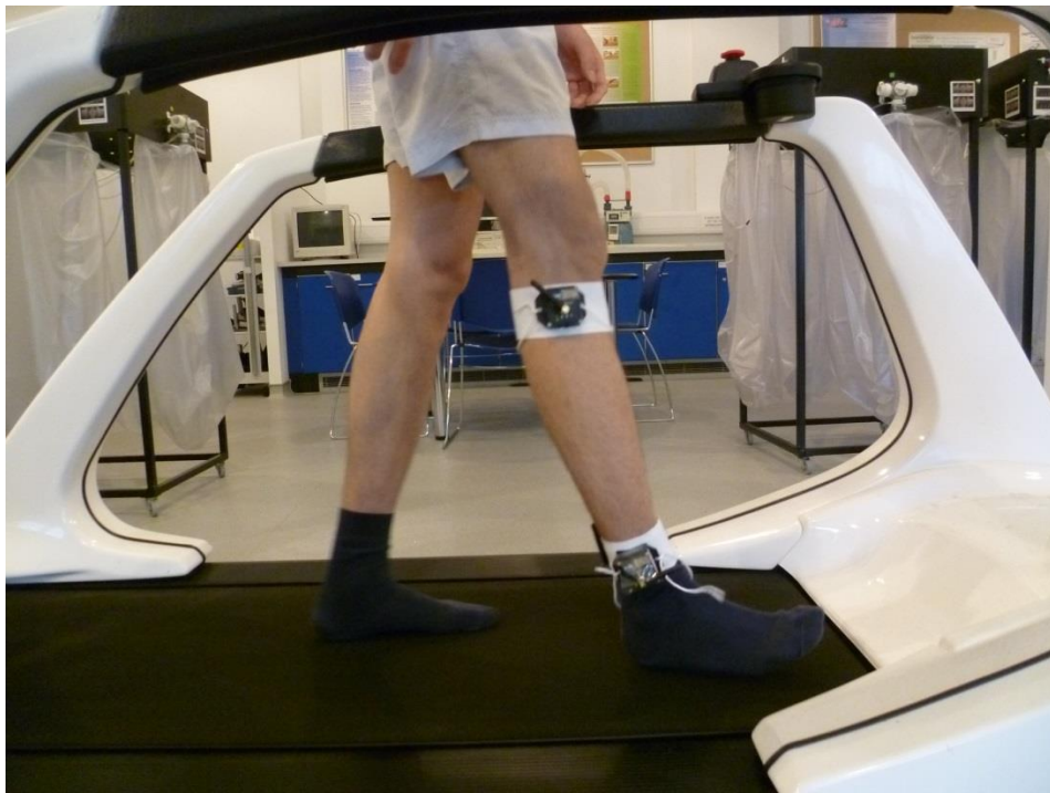
Figure 3.3 A participant walking on a treadmill, with accelerometers mounted on the knee and ankle.
