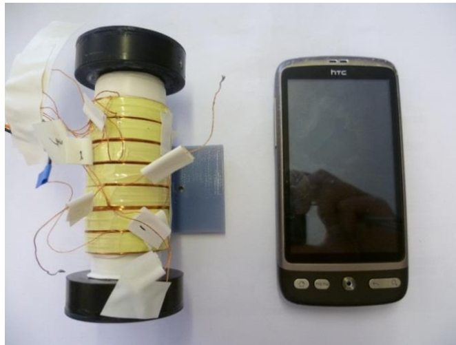
Figure 5.27 Prototype of the magnetic-spring electromagnetic generator alongside a cell phone with a height of 119 mm and a width of 60 mm.
