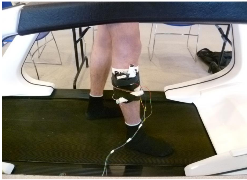
Figure 6.18 A participant standing on a treadmill, with the 2-DOF energy harvester and the accelerometer mounted on the middle of the knee with 0^\circ rotation.
