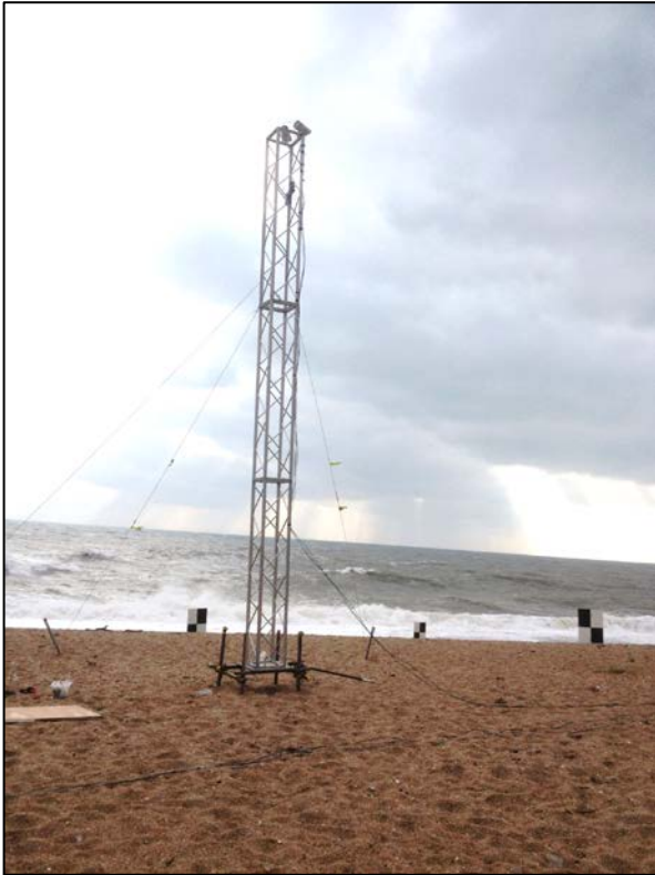
Figure 2: An example of a mobile Argus station deployed by Plymouth University at Slapton Sands for a short field experiment. Two cameras are mounted on a scaffold rig. Checkerboards are placed on the beach, within the cameras field of view to act as ground control points (Photo: S. Pitman).
