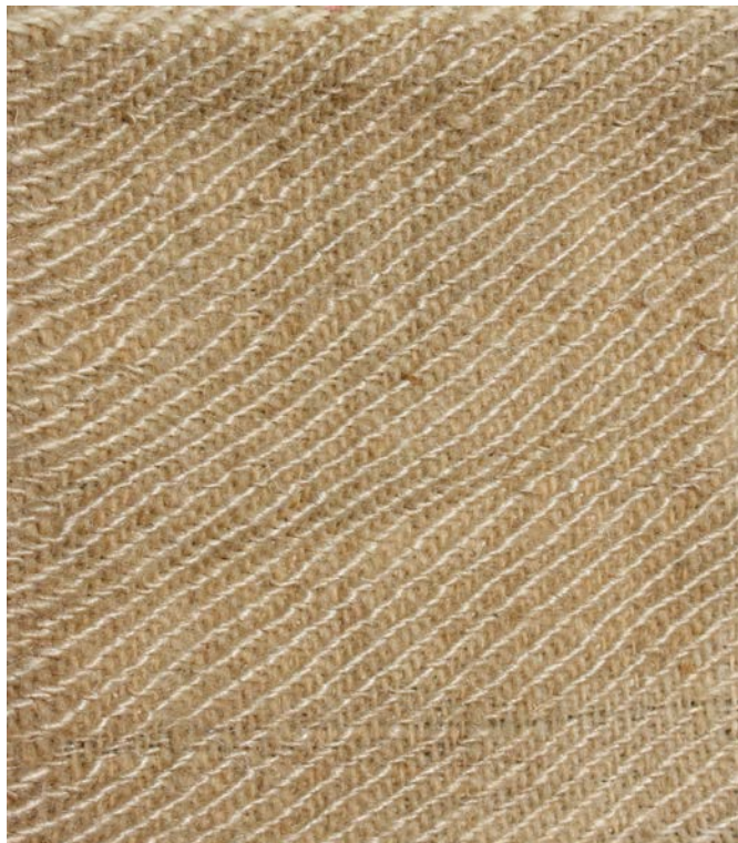
Figure 14: A grey state 2:2 twill, worsted warp and silk weft.
