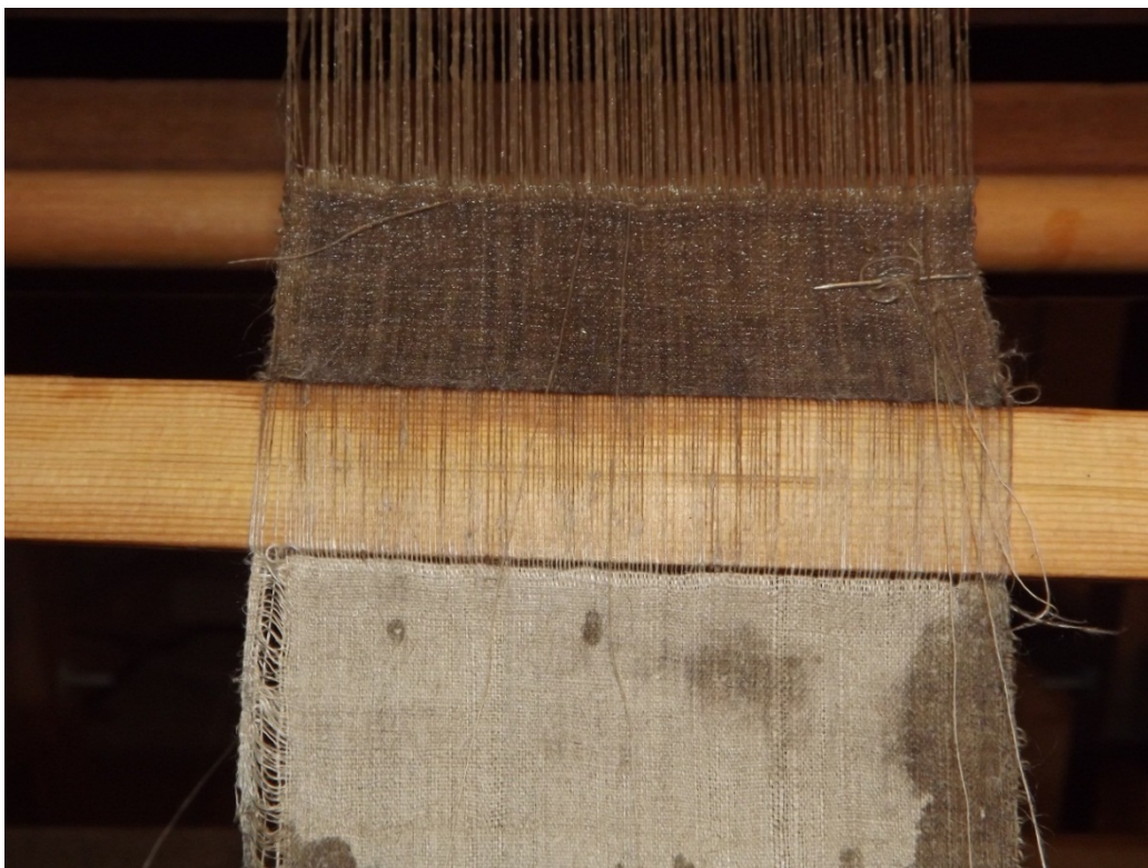
Figure 21: Linen 40's, hand woven on a 4 shaft table loom, demonstrating the amount of water which was needed to maintain the ability to weave.
