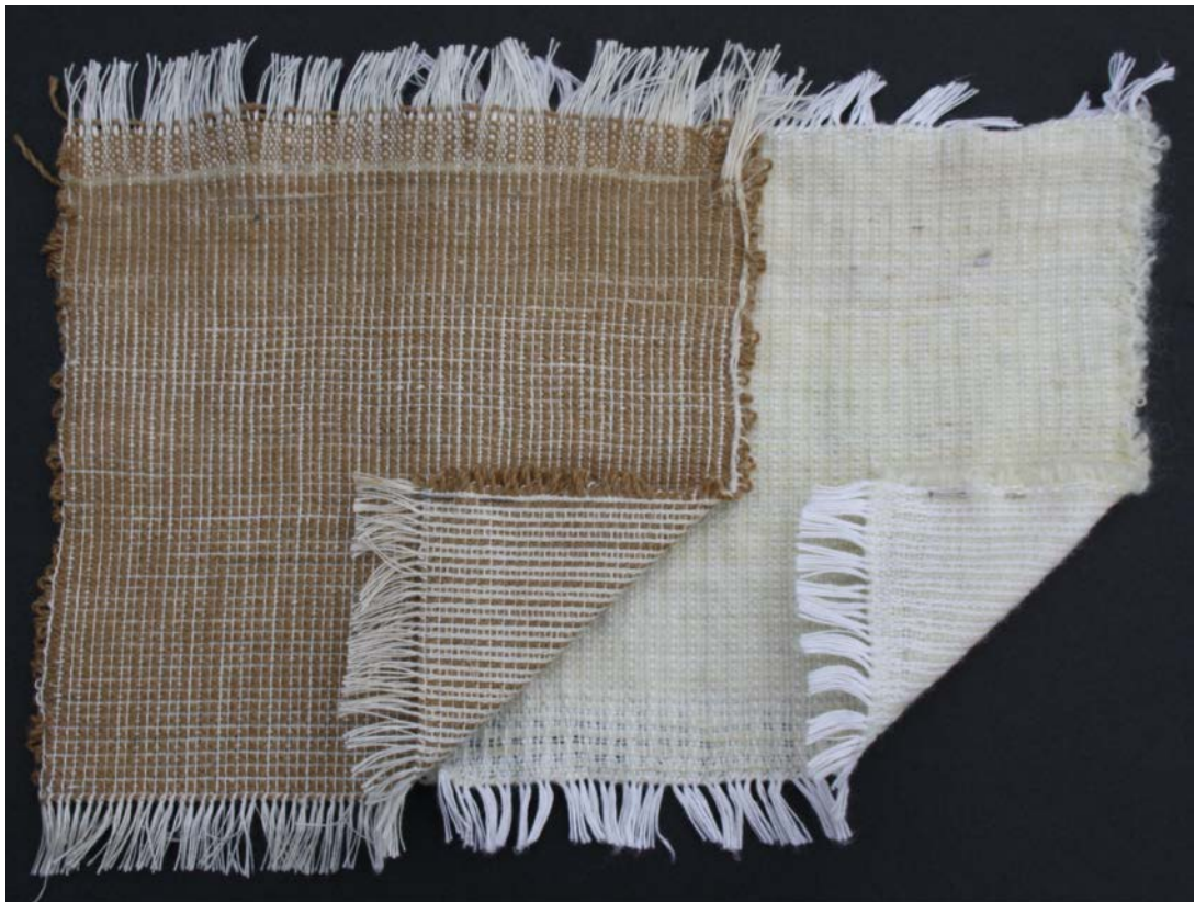
Figure 20: Fustian: Linen warp with weft of Cashmere and linen binder (left). Linen warp with weft of Romney woollen and Romney worsted binder (right).
