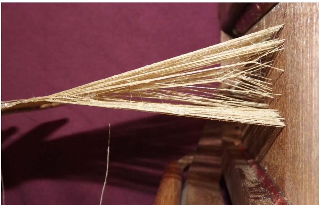
Figure 22: A shed made with the warp dry; illustrating how the fibres all became attached to each other and when the reed was drawn back the strain on the threads resulted in breakages. The water greatly reduced this problem.
