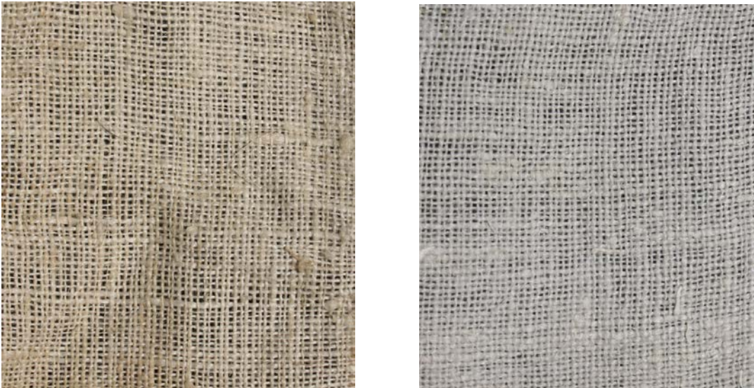
Figure 13: balanced open weave possibly that of a Buckram . linen warp and linen weft. Left: in grey state. Right: washed fulled version.
