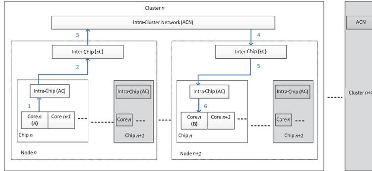
**Fig. 4.** Communication network flow C for message passing between processors on different nodes but within the same cluster.
