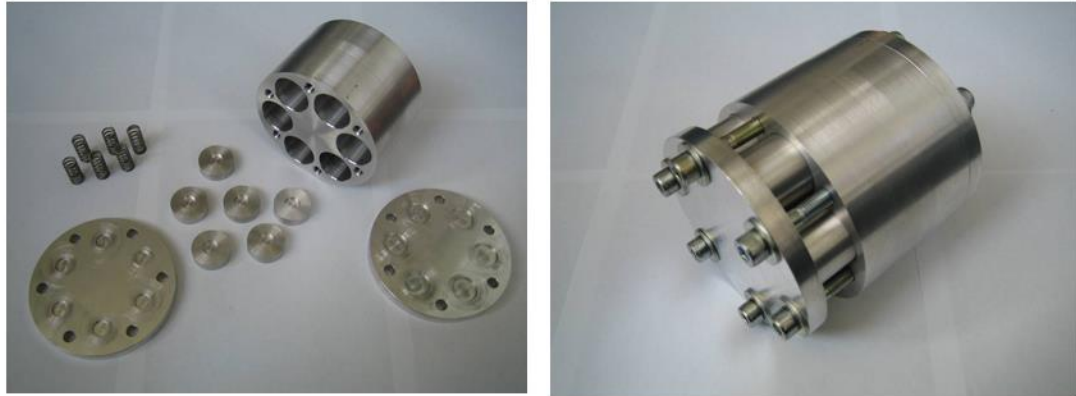
Figure 61: Sample bonding curing jig shown disassembled (left) and assembled containing specimens and mating cylinders (bottom).
