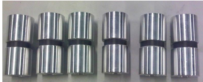
Figure 62: A batch of specimens bonded using FM1000 to aluminium mating cylinders.
