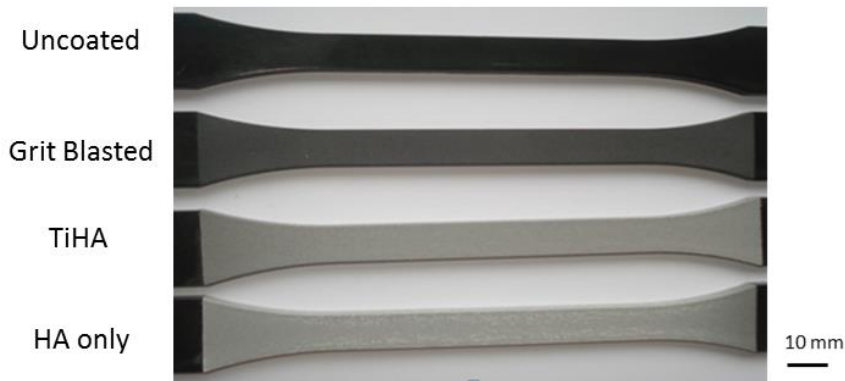
Figure 51: CFRPEEK MOTIS tensile and fatigue specimens according to BS EN ISO 527-1:1996.
