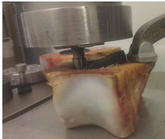
Figure 176: Test setup of edge loading experiment on the implanted components to investigate their primary stability.
