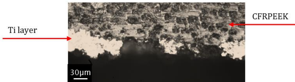
Figure 64: Ti coated specimen where no FM1000 adhesive remained on the surface. The Ti layer partially remains on the surface.
