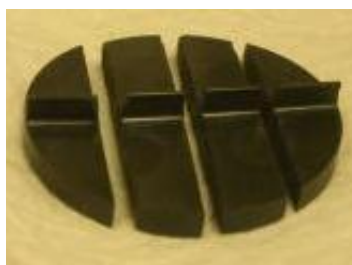
Figure 89: Upstanding Beam MOTIS CFRPEEK specimen cut into 7.5 mm wide specimens.
