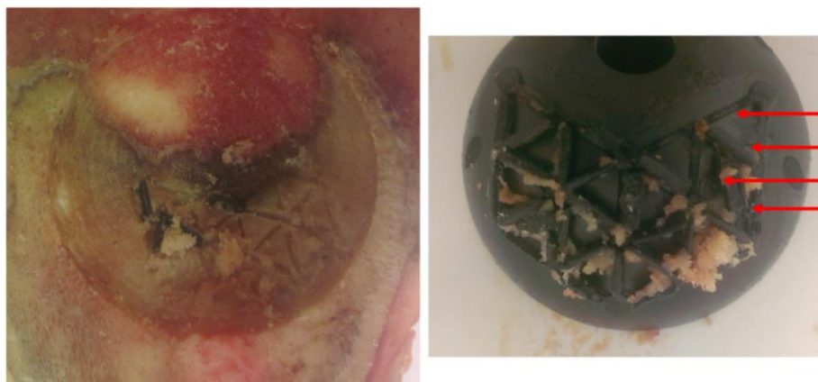
Figure 177: The condition of the implanted bone and injection moulded component after extraction of each component from the 53 and 54 mm cavities.
