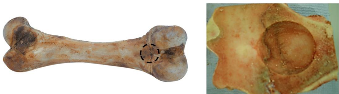
Figure 151: Site of reamed cavity on bovine femur (left) and reamed cavity in section of femur prepared for CFRPEEK implantation.
