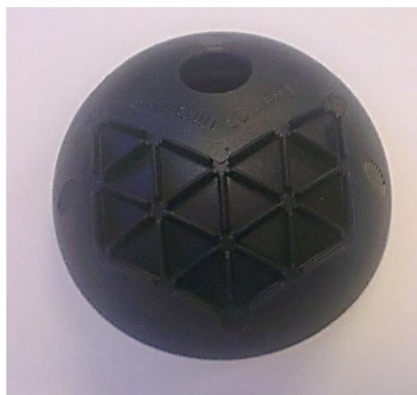
Figure 98: CFRPEEK acetabular cup from which upstanding beams were individually removed.
