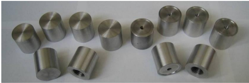
Figure 60: Aluminium mating cylinders for specimen mounting. Coating face cylinders on the left and back face cylinders on the right (Note recess for specimen alignment).
