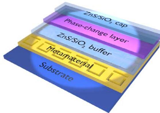
The combined device results in a tuneable metamaterial that can be reversibly switched to different resonant frequency states through optical crystallisation or amorphisation of the phase-change layer. The device can obtain effective refractive index changes impossible in conventional, unstructured materials, and has applications as an all-optical light modulator with a tuneable operational wavelength and a memory of its previous state<sup>3</sup>.
