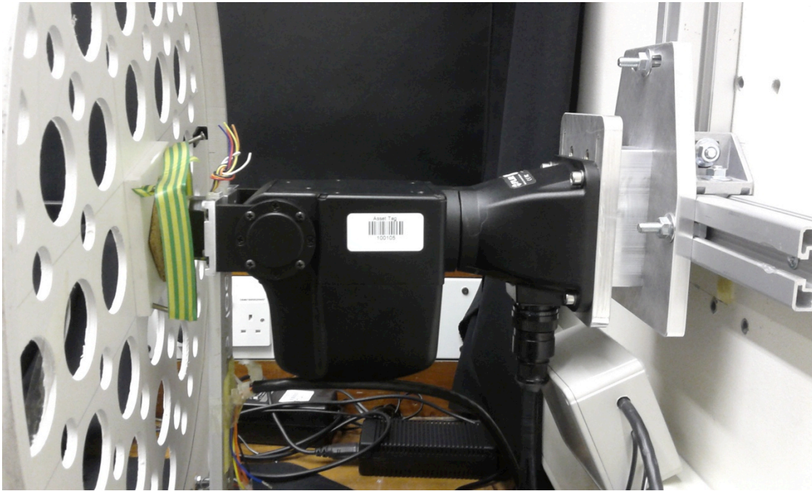
Figure 0.4. PTU mounted to wall (shown rotated from home by 90). Mounting bracket allows entire unit to be shifted left/right or up/down if desired. Stimulus surface (shown from behind on the left) is 40cm from the wall at frontoparallel. Cable boxes are stuck to the wall to avoid collision with the surface as it rotates.
