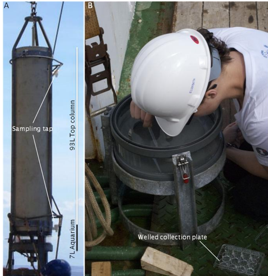
Figure 3-2. The 100L Marine Snow Catcher (A) and the particle collection technique (B): each particle was transferred from the aquarium to an individual well in a welled plate using a glass Pasteur pipette.
