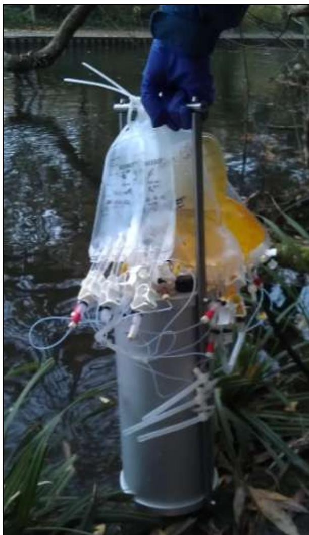
Figure 5-8 – P2 device in housing on the River Beaulieu shore, before deployment. Reagents and waste storage bags are shown attached to the external frame of the device.
