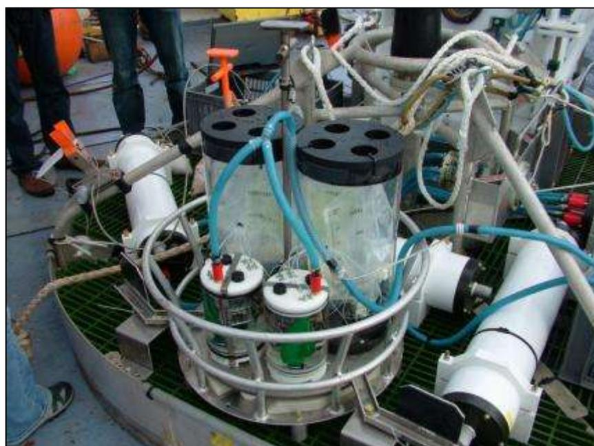
Figure 3-10 – Iron analysers on SEAMON-EST platform. Deployment set up. *Pourquoi Pas?* main deck.
