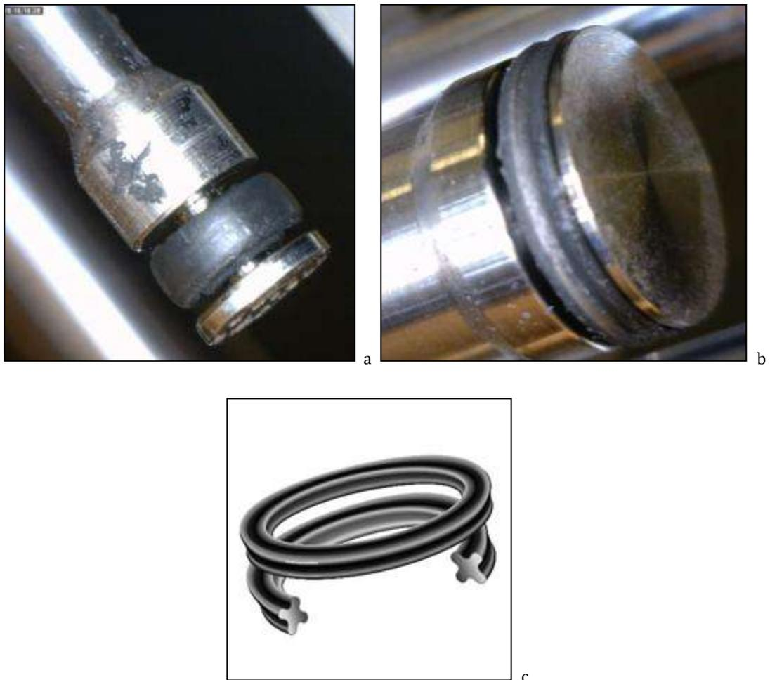
Figure 3-15 – Picture of worn out pump's Viton quad-rings. a) Quad-ring on small syringe plunger. Plunger size: 3.30 mm x 12.4 mm (maximum stroke). b) Quad-ring on big syringe plunger. Plunger size: 9.69 mm x 12.4 mm (maximum stroke). c) Drawing of the original shape of the quad-rings.
