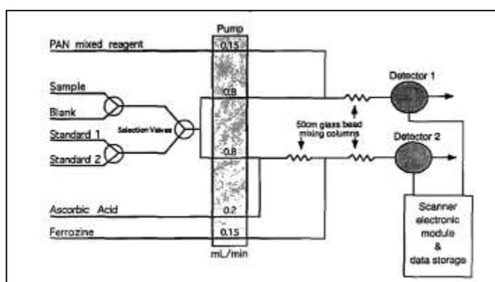
Figure 1-3 – SCANNER manifold configuration for the determination of dissolved Mn and total dissolved Fe in-situ. From (Chin et al. 1994).
