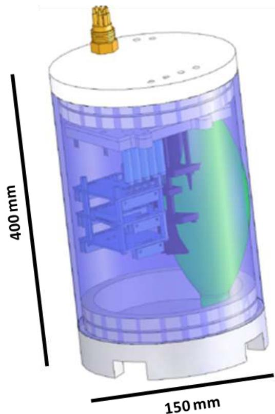
Figure 3-5 – The analyser enclosed in the clear plastic cylindrical housing. In green is the pressure compensating bladder, over-expanded. On the top end cap are the the bulk head connectors. Fluidic connectors are not shown. Idea and CAD drawing by Dr. C.F.A. Floquet.
