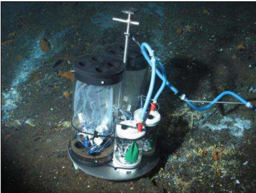
Figure 3-11 - Module of two Fe(II) analysers positioned on a diffuse flow vent site. Two small cylinders (400 mm x 150 mm): chemical analysers. Two big cylinders (800 mm x 250 mm): plastic housings for reagents/standards and waste storage bags. The cable for power and communication connection to SEAMON-EST is also visible. Photo: Victor 6000, Ifremer, France.
