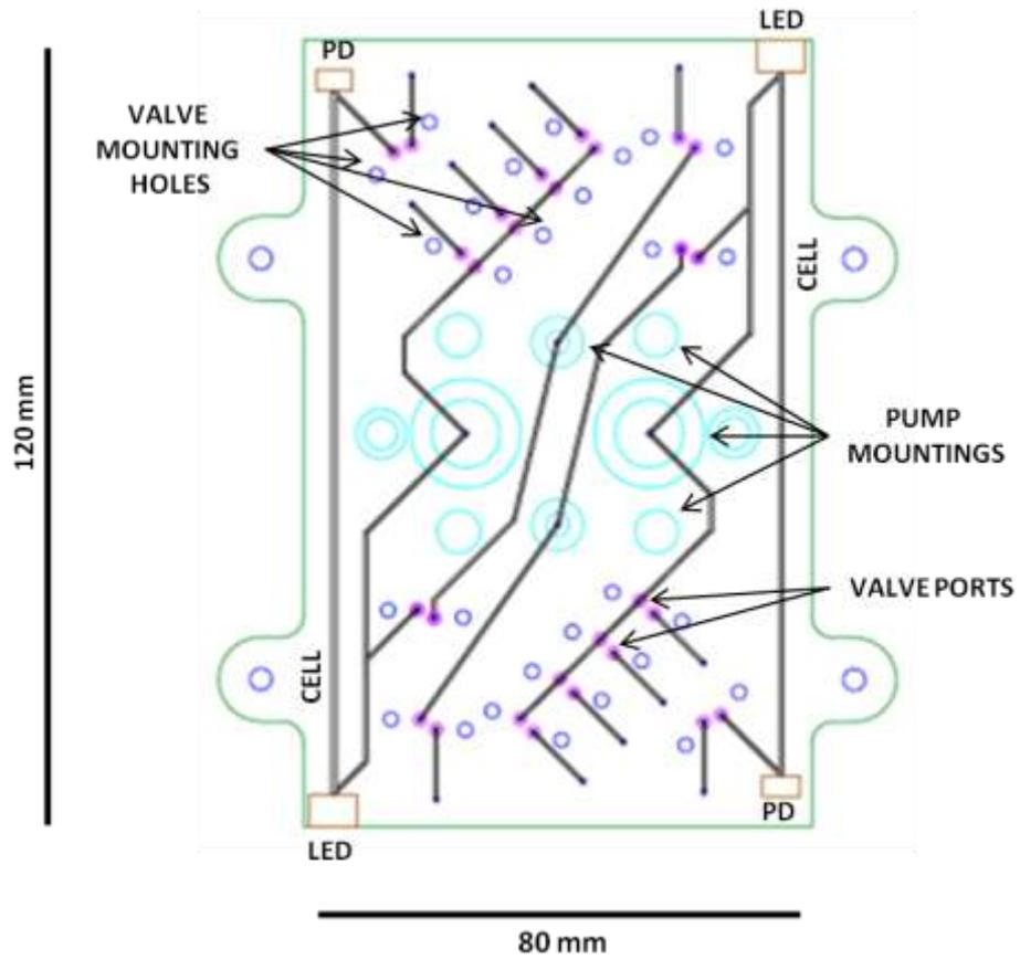
Figure 4-4 - CAD drawing of the microfluidic chip showing external shape (green), location of LEDs (large orange rectangles), photodiodes (small orange rectangles), recesses for pump mountings (turquoise), microfluidic channels (black), valve ports (pink), and mounting holes (indigo).
