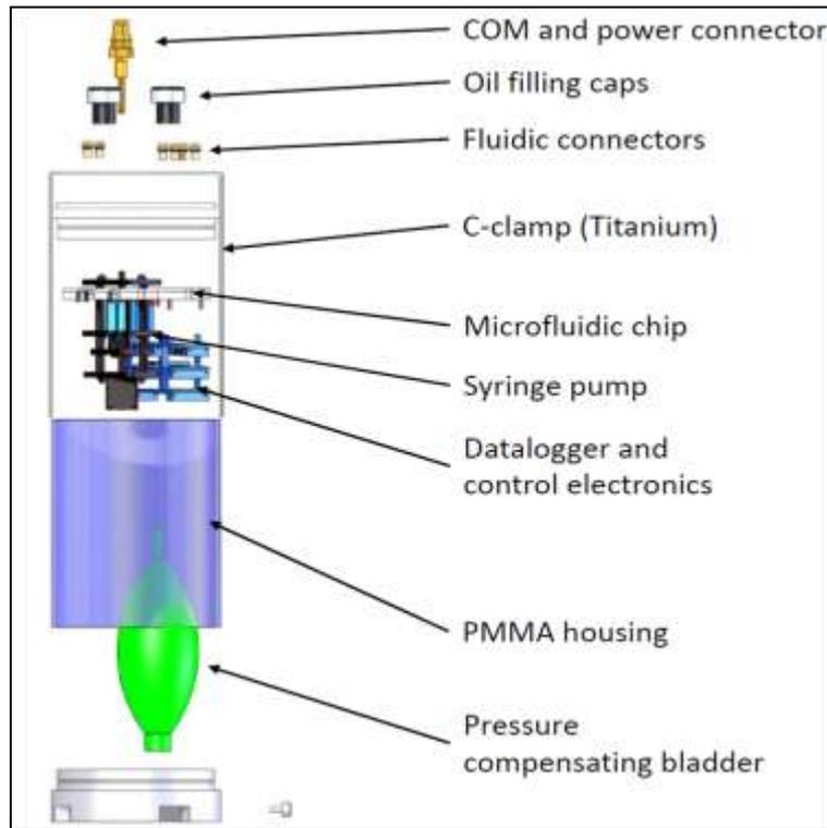
Figure 3-6 – Exploded view of the analyser in the pressure compensated housing. CAD drawing by Dr. C.F.A. Floquet.
