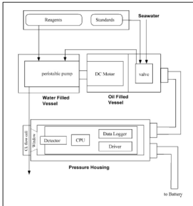
Figure 1-5 – Schematic of GAMOS Mn analyser. From (Okamura et al. 2001).
