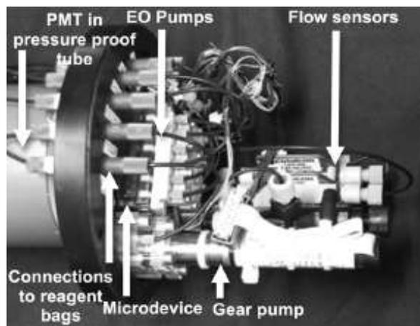
Figure 1-10 – IISA-Mn setup on ROV. (Provin et al. 2013)
