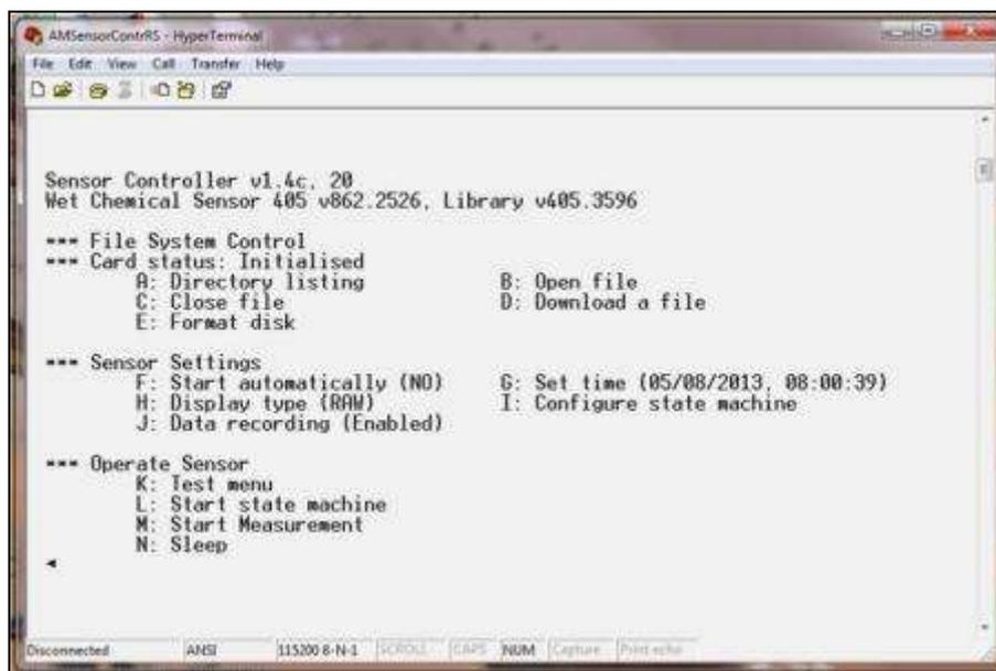
Figure 3-3 – Screen-shot of the user-sensor interface used to control the sensor’s operations.
