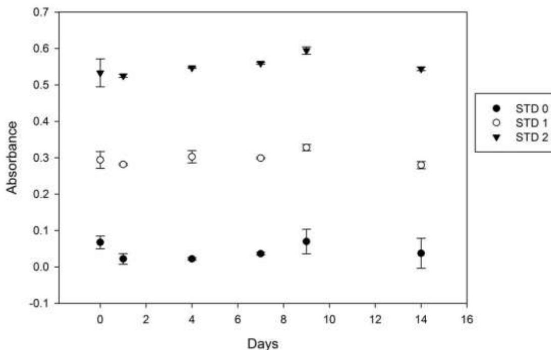
Figure 2-2 - Long-term experiment to test the stability of the PAN-Desferrioxamine reagent over time. STD 0: 0  $\mu\text{M}$  Mn; STD 1: 1  $\mu\text{M}$  Mn; STD 2: 2  $\mu\text{M}$  Mn.
