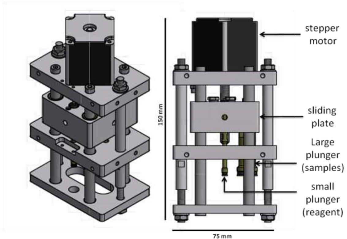
Figure 3-4 – CAD drawing of the custom-made syringe pump. Top and side view. In the picture can be seen the stepper motor driving the sliding plate and the two (small and large) plungers. The barrels covering the plungers are not shown. Idea and drawings by Dr. Ed Waugh, Sensors Group, NOC, Southampton.
