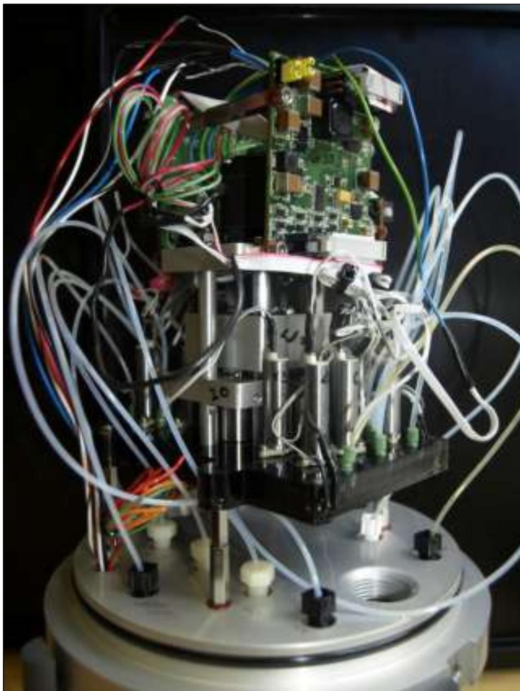
Figure 4-9 – PMMA microfluidic chip P2 with fluidic connectors, LEDs, photodiodes, valves, syringe pump, electronics boards and tubing, mounted on anodised aluminium housing end-cap, before being put into the cylindrical housing.
