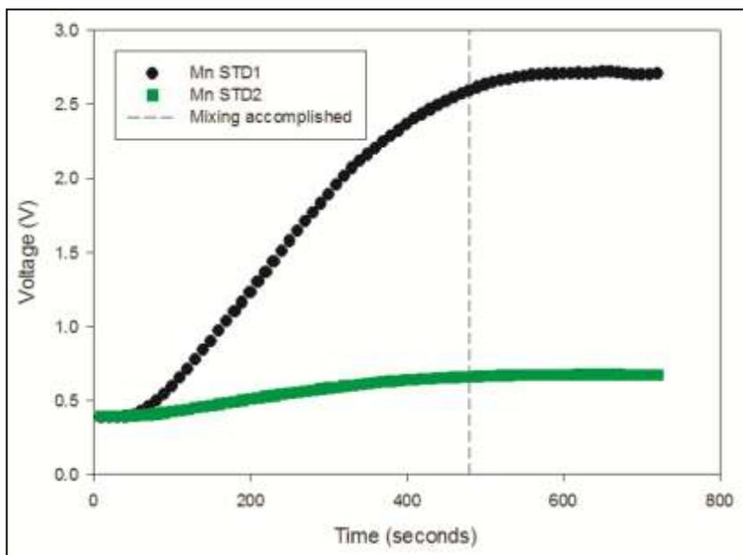
Figure 4-3 – Mn and PAN diffusion time test for mixing across a 600  $\mu\text{m}$  wide x 100 mm long cells under no-flow conditions. Temperature 20°C. Standards prepared in Milli-Q water matrix. The dashed line indicates when the analyte and reagent solutions are fully mixed and reacted. Mn standards 4.55  $\mu\text{M}$ , 9.1  $\mu\text{M}$ . Test was performed directly on Prototype 2. The voltage output of the sensor with time is shown.
