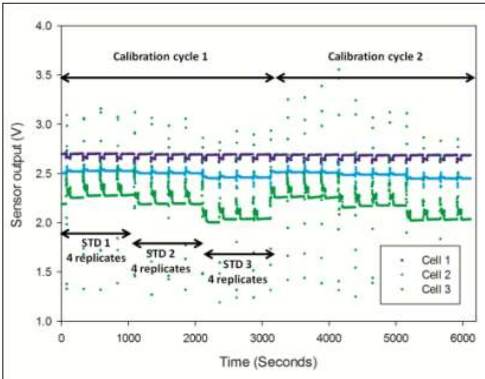
Figure 3-9 - Raw voltage output of the Fe(II) analyser during 2 calibration cycles.
