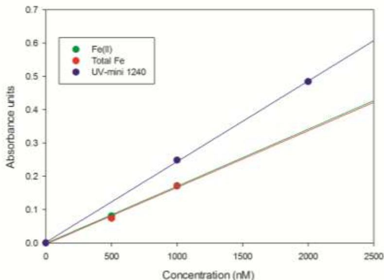
Figure 4-12 – Fe(II) and Total Fe calibration curves compared to calibrations obtained with a Shimadzu UV-Mini 1240 Spectrometer. Fe(II) standards: 0 nM, 500 nM, 1000 nM, for the analyser; 0 nM, 1000 nM, 2000 nM, for the bench top spectrometer.
