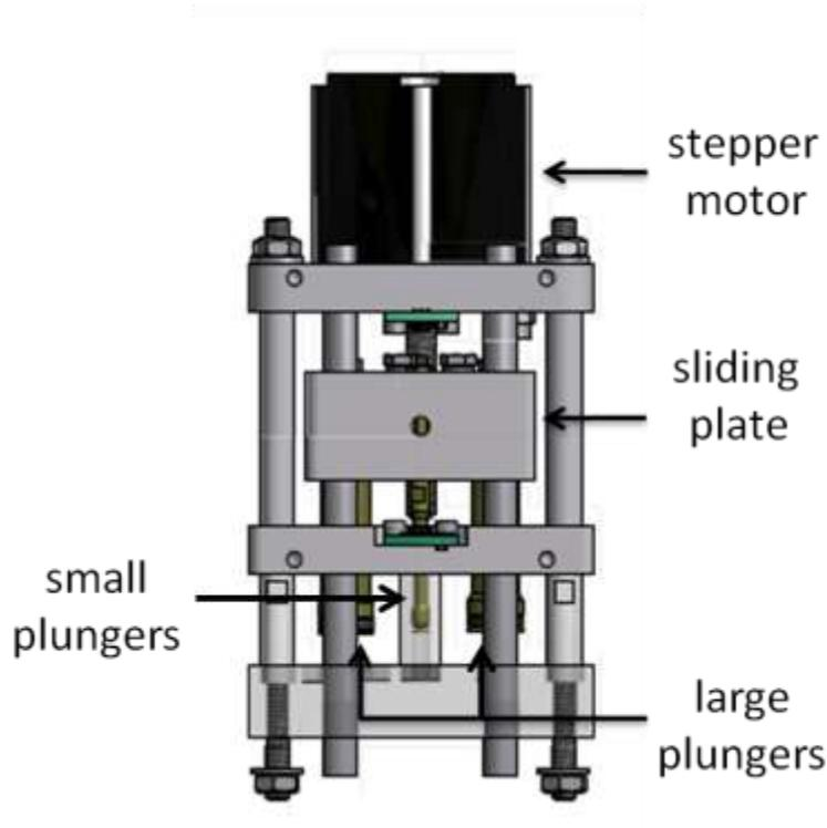
Figure 4-6 - CAD drawing of the second version of the custom-made syringe pump. Front view. The two large plungers are clearly shown, while the second small plunger is hidden behind the first one. Idea and drawings by Dr. Ed Waugh, Sensors Group, NOC, Southampton.
