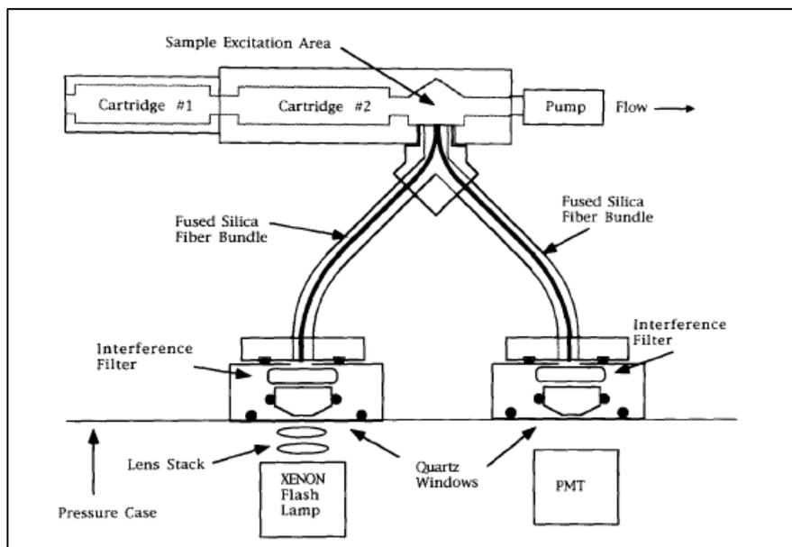
Figure 1-4 – Schematic of the ZAPS fiber optic spectrometer. From (Klinkhammer 1994)
