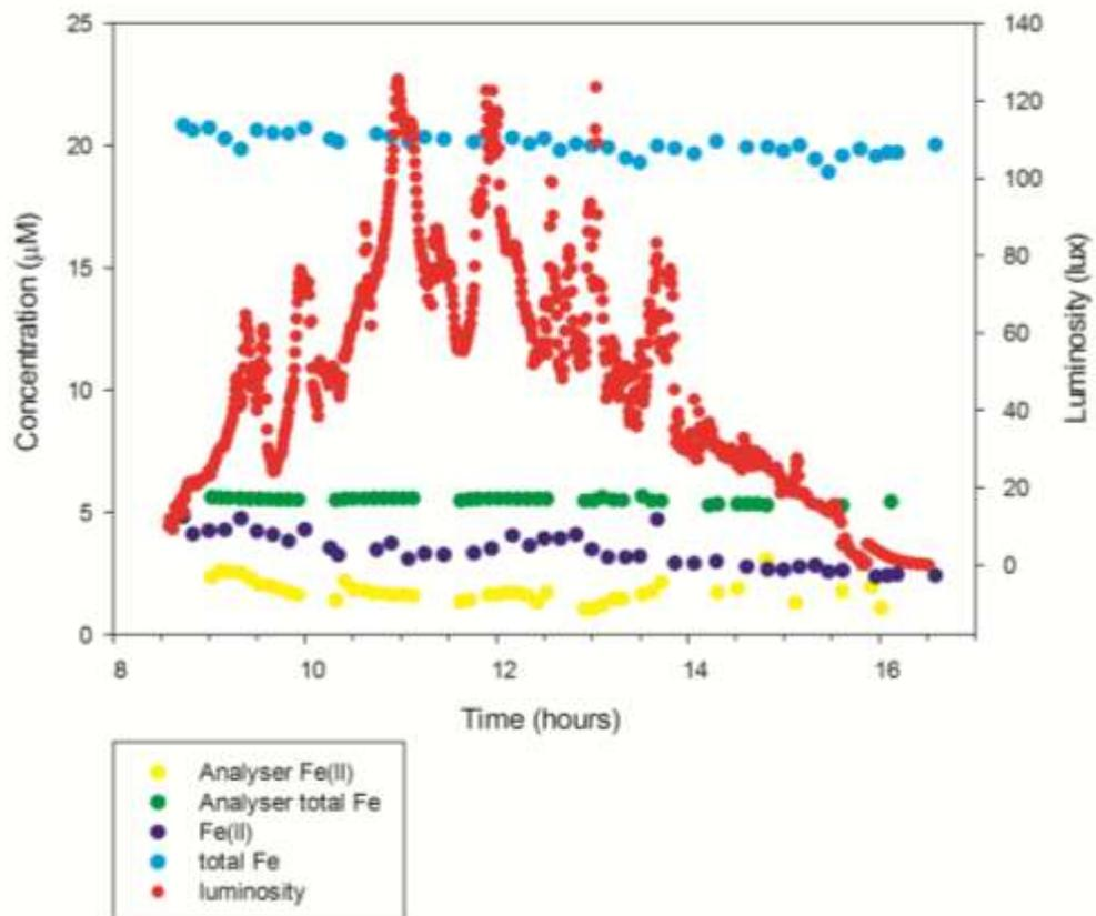
Figure 5-9 – 17-12-12 - King's Hat footbridge, River Beaulieu, Southampton, UK. Luminosity data; Total Fe and Fe(II) data obtained from in-situ measurements and manual sampling. Data recorded from 1 hour prior to sunrise until 1 hour after sunset.
