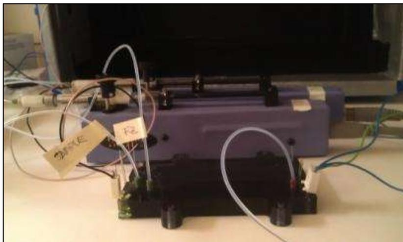
Figure 4-1- Diffusion time tests set up. For this test a new purpose built chip was used. The test-chip is shown attached to the syringe pumps for the injection of sample and reagent.
