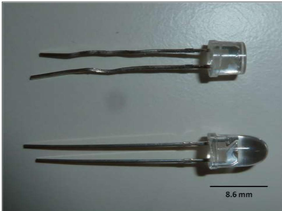
Figure 4-8 – A flattened LED and a dome shaped one. The flat surface allowed more light to reach the photodiode at the other extreme of the optical cell than the curved surface.
