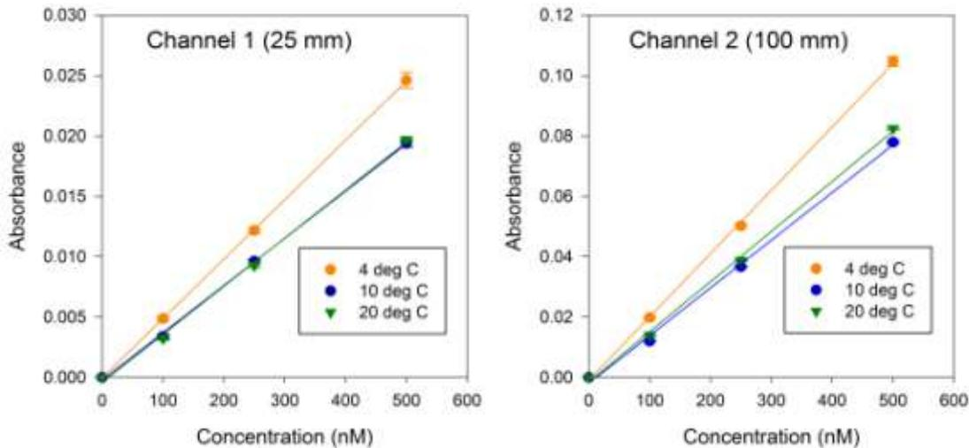
Figure3-12- Calibration at different temperatures, Channel 1 (25 mm) and Channel 2 (100 mm) results shown separately.
