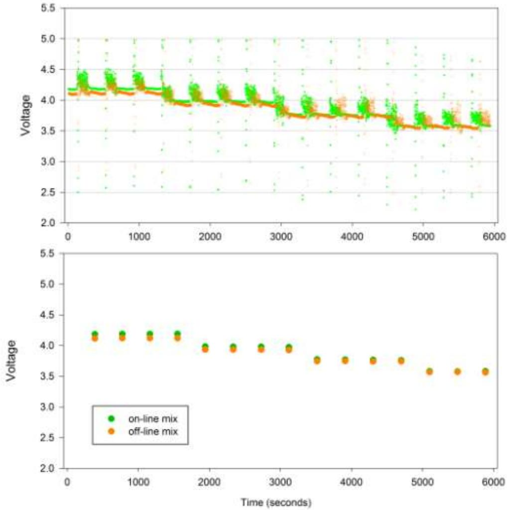
Figure 3-2 – Raw voltage output of the Fe(II) analyser for 0 nM, 100 nM, 250 nM, 500 nM Fe(II) Standards..
