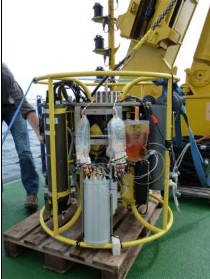
Figure 5-3 -Analyser attached to the IOW-Pump-CTD
