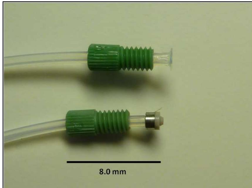
Figure 4-7 – Top: microfluidic connector with flanged tubing edge as gasket (used on P2). Bottom: microfluidic connector with stainless steel compressor ring and plastic nipple (used on P1). The green plastic nut sits against the flange or the ring.
