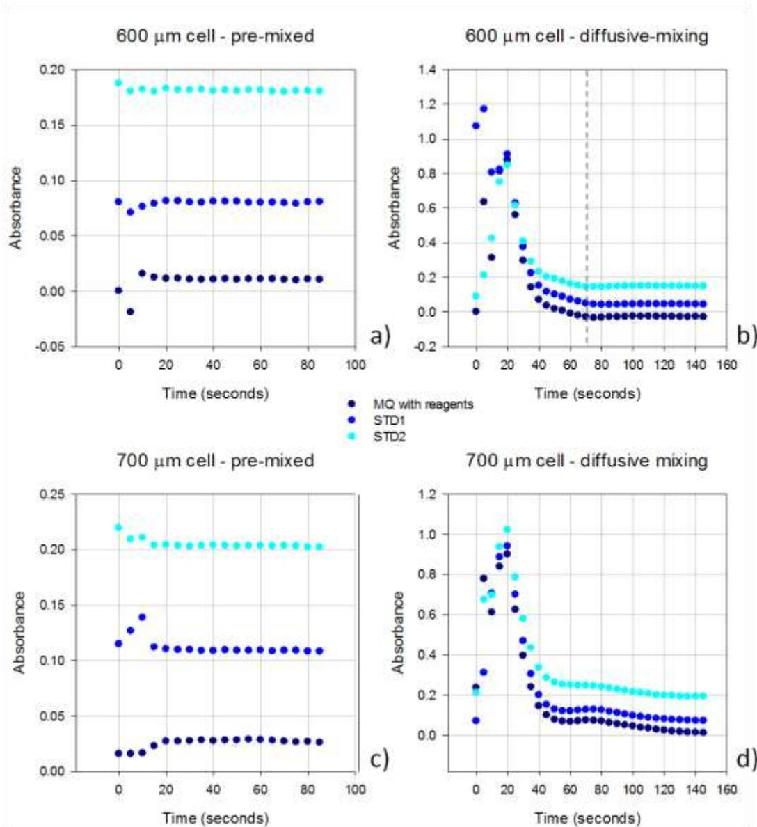
Figure 4-2 - Fe(II) and FZ diffusion time tests for mixing across a 600 μm and a 700 μm wide x 100 mm long cells under no-flow conditions. Temperature 20°C. Standards prepared in Milli-Q water matrix. The dashed grey line in plot b) indicates when the analyte and reagent solutions are fully mixed and reacted. Standards 0.5 μM, 1.0 μM.
