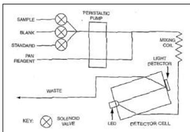
Figure 1-8 – Schematic of Statham et al. in-situ Mn analyser manifold. From Statham et al. (2003).
