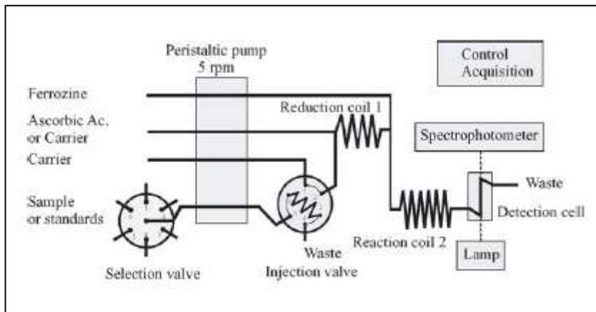
Figure 1-7 – Schematic of ALCHIMIST Fe analyser. From (Sarradin et al. 2005).
