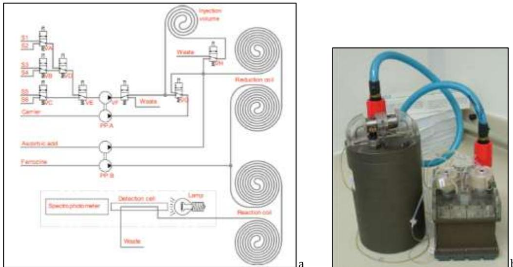
Figure 1-9 – a. Schematic of CHEMINI manifold. b. Integrated system ready for deployment. From (Vuillemin et al. 2009).
