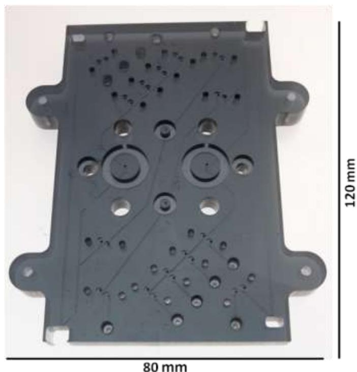
Figure 2-3 - A bonded chip in which optical channels have been machined (chip made by A. Milani).
