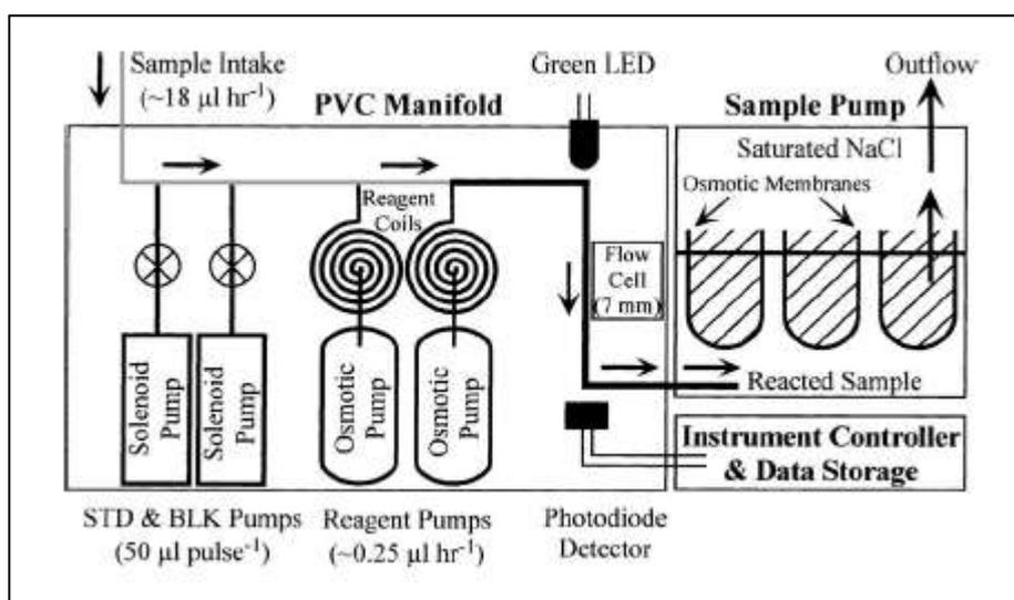
Figure 1-6 – Schematic of Fe-Osmo analyser. From (Chapin et al. 2002).
