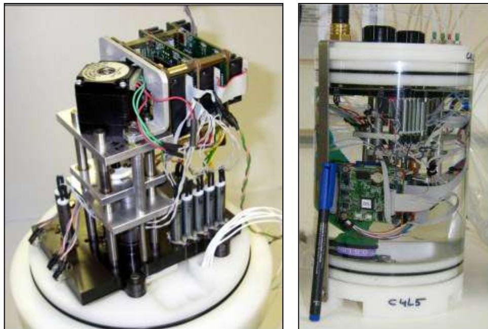
Figure 3-7 – Photographs of assembled analyser outside and inside the pressure compensated housing.
