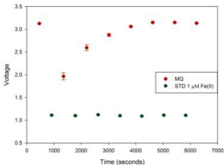
Figure 4-10 - Flushing test. Every point averages 50 measurements of MQ and 1  $\mu\text{M}$  Fe(II) standard. Errorbars on graph.
