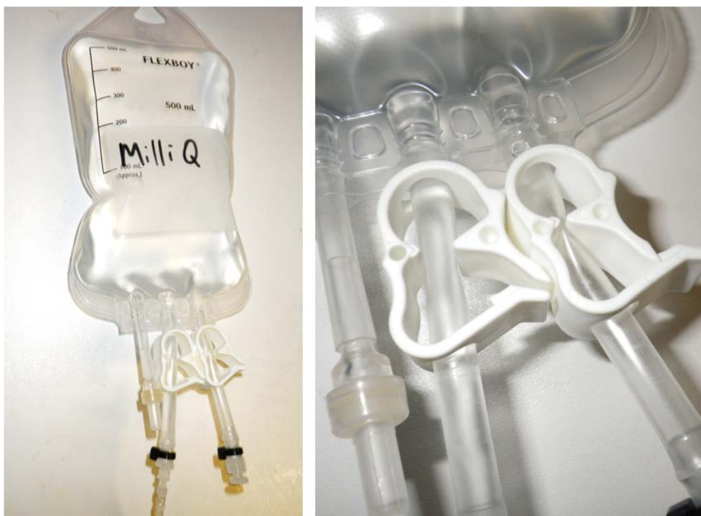
Figure 4-10 - Sample storage bag similar to the one used for alkalinity measurement. The close up shows one clip open, one closed.
