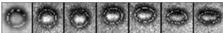
FIG. 4. Images showing a single osmotically swollen red blood cell under the influence of a range of acoustic pressure amplitudes from 0–978 kPa (going left to right). White line shows fitted ellipse.
