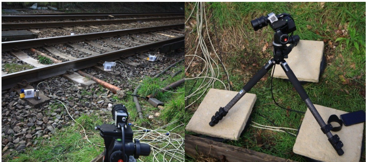
Figure 8: (a) targets on sleepers and (b) camera set up
