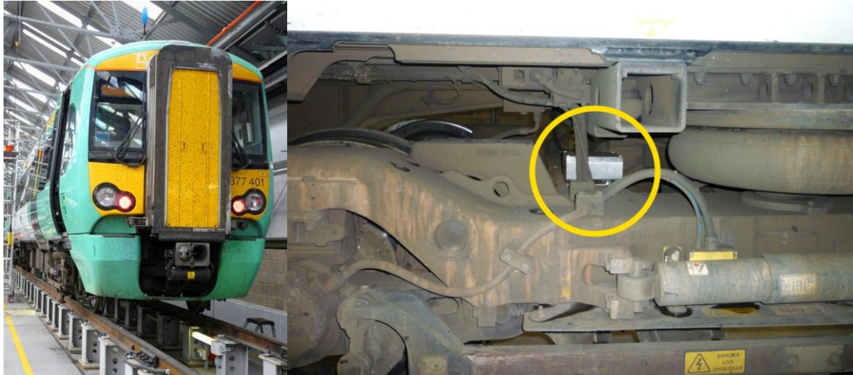
Figure 9: Class 377 train and location of inertial measurement box
