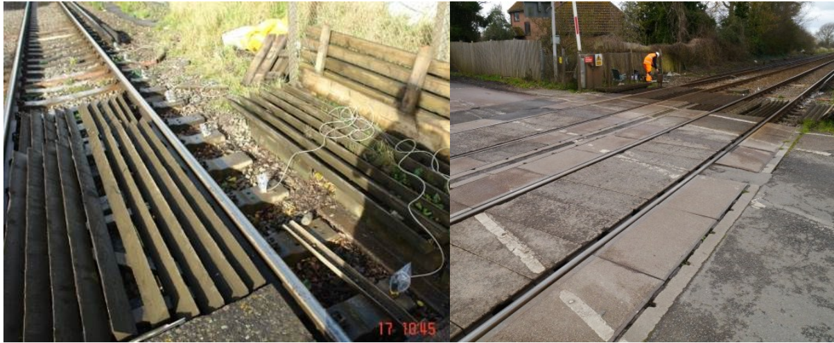
Figure 5: (a) Arrangement of geophones and (b) level crossing viewed from the opposite side of the road from the instrumented section
