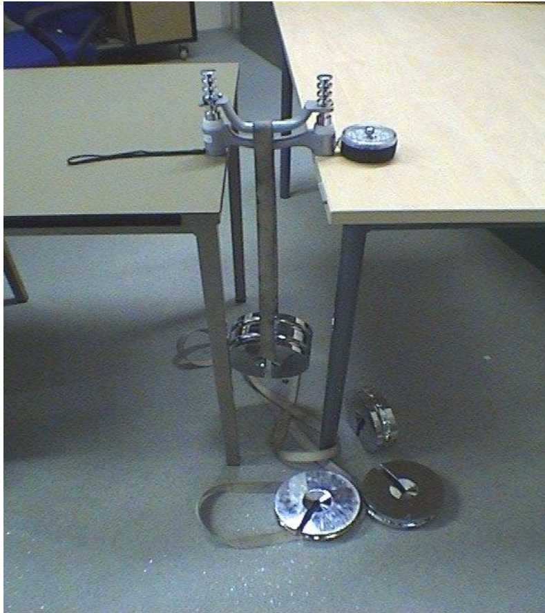
Figure 2.8 Assessing the accuracy of the Jamar against known weights
