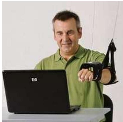
**Figure 7.1 Armeo<sup>®</sup> Boom Robot which can be used at the participants' home**
