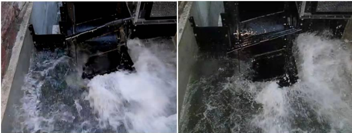
Figure 6.5: Blade splash compared for differing water depths at rotor speeds of 9 rpm: The deeper water condition is on the left.
