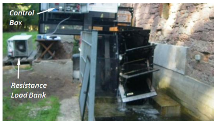
Figure 5.8: Test set up for Load Bank Control.
