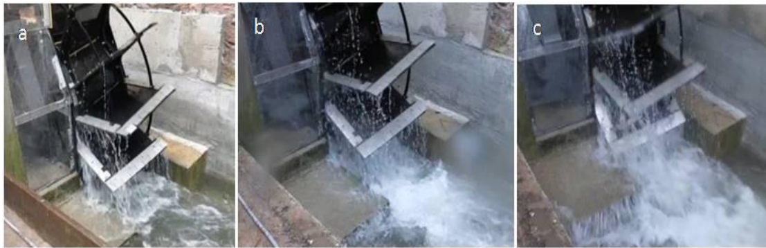
Figure 6.9: Exit Flow Close to the wheel: a. wave formation driven by large variation in flow velocity (5.7 rpm), b. stable hydraulic jump formation at end of panniers (10.5 rpm), c. water spout produced at high flow rates (13.9rpm).
