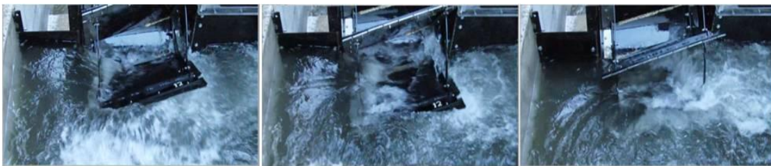
Figure 6.2: Cell Side Filling at 3.7 rpm – fill progresses left to right, Note the creation of asymmetric flow in plenum.
