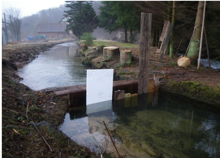
Figure 5.7: Using the Fish Screen to throttle inlet flow during Inverter control tests.
