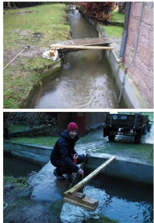
Figure 5.3: a. Velocity Measurement Test section. b. Velocity measurements being carried out by S. Schneider, TU Darmstadt
