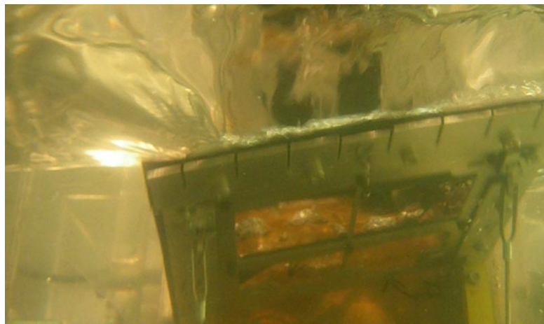
Figure 10.16: 6-Blade Flap Wheel Shortly after Making contact with the upstream surface.
