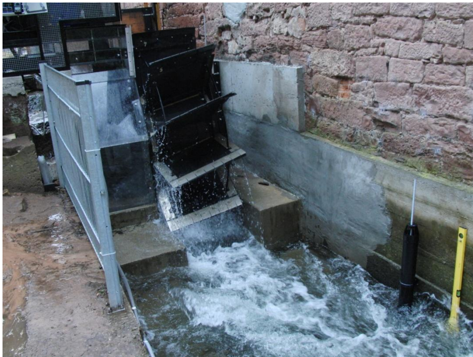
Figure 6.10: Turbulent and asymmetric flow conditions in the exit channel: wheel speed is 8.4 rpm
