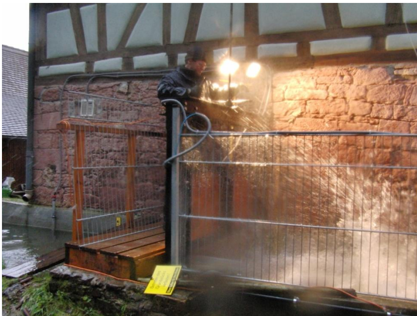
Figure 6.6: The violence of blade splash (shown here at 10.6rpm), made prolonged operation of the machine hazardous, and generation speeds were limited to below 6rpm as a consequence
