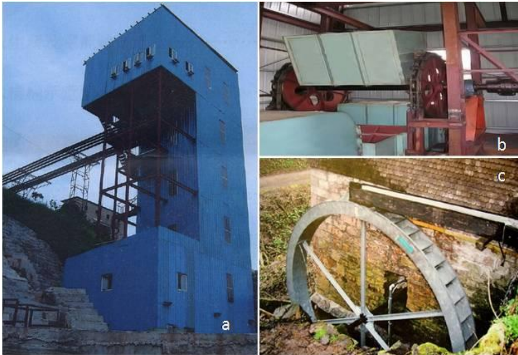
Figure 2.2: Pure Potential Machines: a & b. Yiu Hwa Chain Turbine (Nguyen Minh Duy, 2012), c. Overshot water wheel (HydroWatt).
