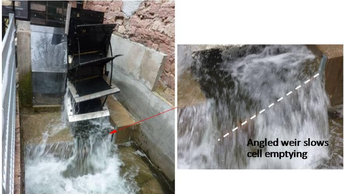
Figure 6.8: Ventilation Reduction Test: an angled weir was added to the end of the side panniers to raise local water levels and reduce the speed of cell emptying. (photo: Jurgen Kunkel)
