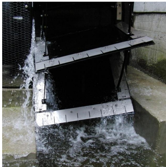
Figure 5.9: Leakage Flows during Static Rotor Test. Note the significant leakage past the hub seals
