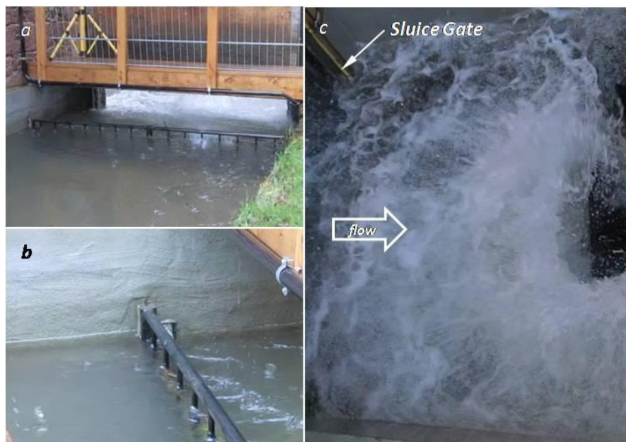
Figure 6.1: Inlet Turbulence at 11.6 rpm – a. Safety screen and gate with plenum visible beyond, b. head drop across safety screen = 20mm, c. Extreme turbulence in Plenum
