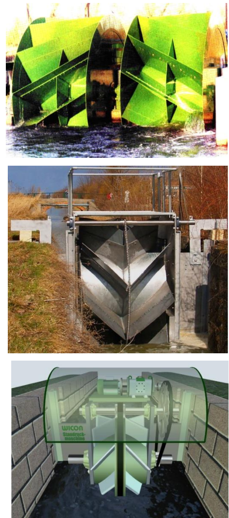
Figure 3.8: The Stem Pressure Machine: (top to bottom), The Mk1 unit, Mk2 installation, speed increaser system (Brinnich 2011)
