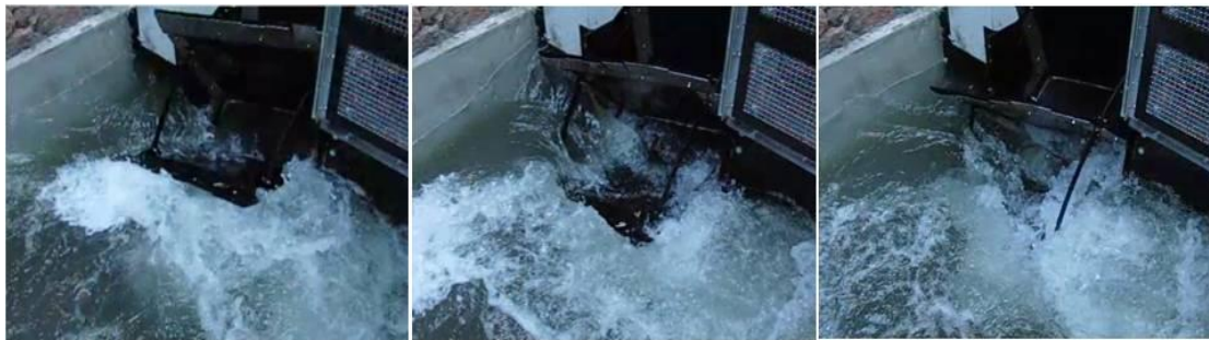
Figure 6.3: Cell Side Filling at 5.7 rpm – initial blade splash is high, forming a steep wave front on the left hand inlet side of the cell. High turbulence is evident as water enters from three sides of the blade.
