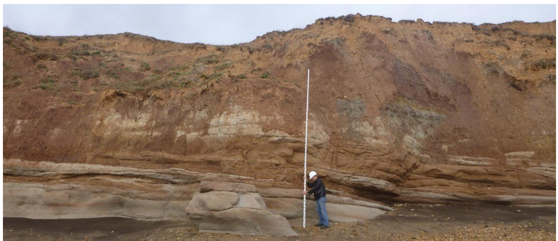
Figure 4.6: An example of a steep cliff with high level sliding (CBUC) in the Wessex Formation to the south eastern end of the Sudmoor Point Sandstone. The measuring staff is 5m long. (Source: Original Photograph).
