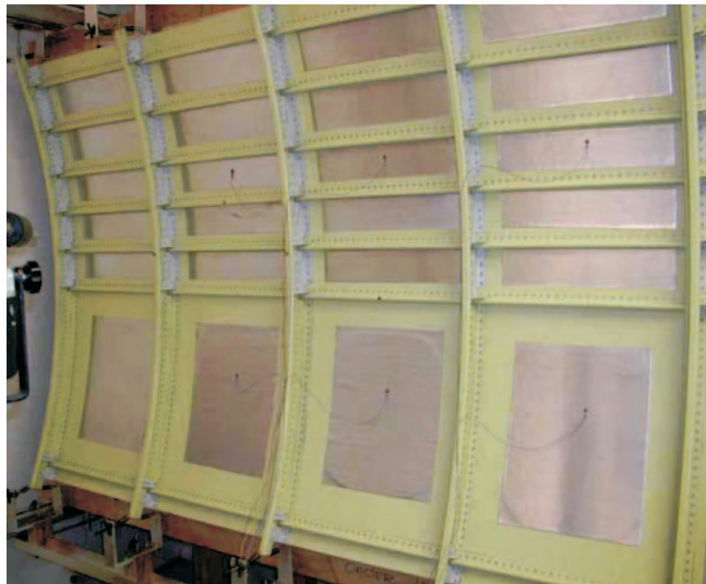
Figure 1.4: Fuselage panel added with damping material [16].
