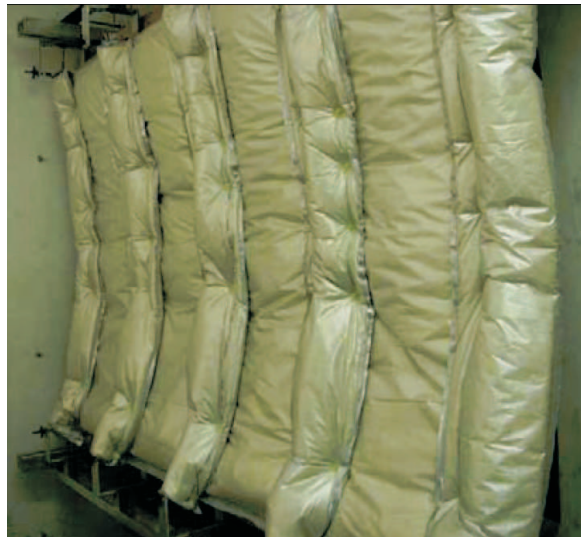
Figure 1.2: Fuselage panel added with bagged fiberglass blanket [16].
