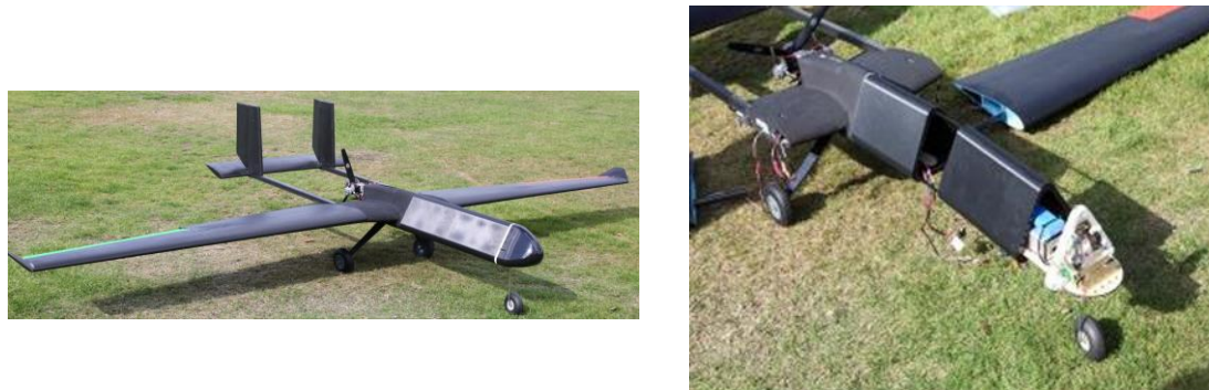
FIGURE 5-2: DECODE UAS SHOWING MODULAR APPROACH. REPRODUCED WITH PERMISSION FROM ANDY J. KEANE 3 .
