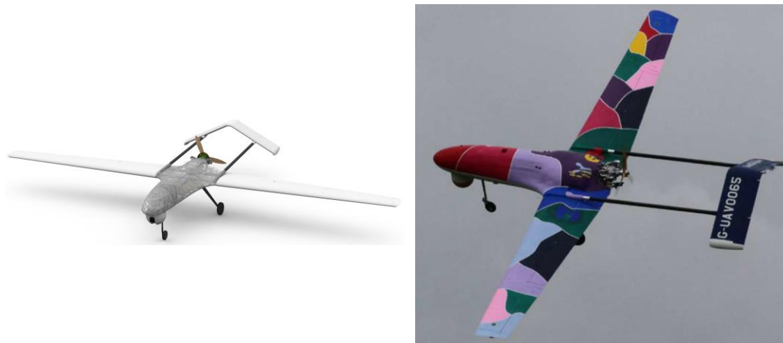
FIGURE 5-3: BBC UAS VIRTUAL DESIGN (A) AND ASSEMBLED AIRCRAFT INFLIGHT (B). REPRODUCED WITH PERMISSION FROM JEROEN VAN SCHAIK 4 AND ANDY J. KEANE 5 .
