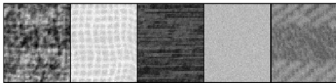
FIGURE 5.37: The visual factor filters, C_{if} learnt from the 64 \times 64 size patches of Brodatz data set. The learnt filters resemble the texture strokes showing the capability of learnt filters to detect local texture patterns.
