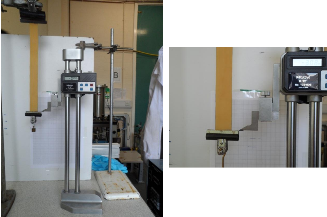
Figure 4.23: Membrane deflection measured by height gauge
