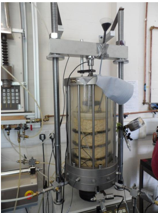
Figure B.3: Resin being poured into the specimen 'T7'
