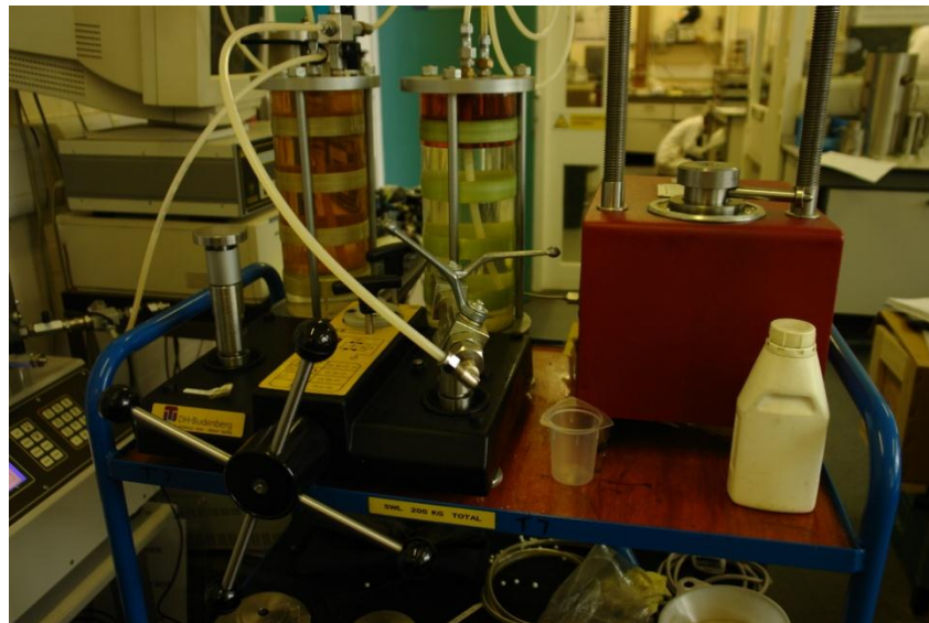
Figure 4.3: Calibration frame- Budenberg S/No 26494/500
