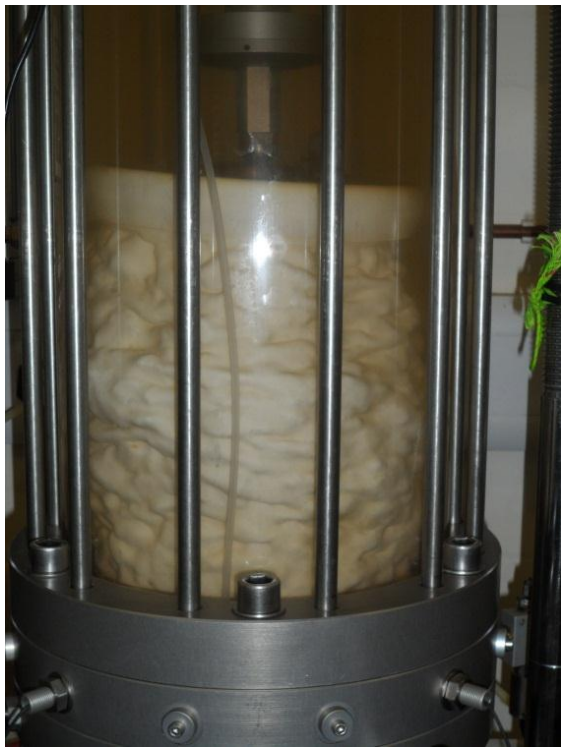
Figure 5.3: Specimen after shearing of 15 kPa saturated test
