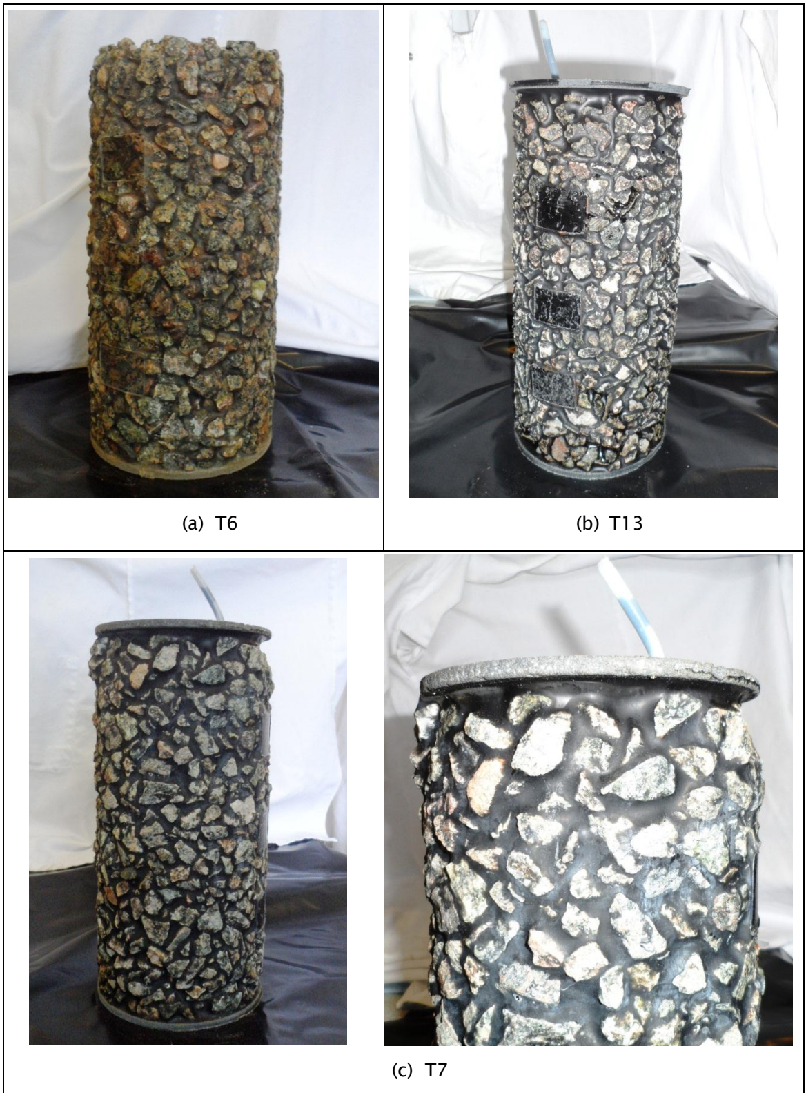
Figure B.4: Resin stabilization of triaxial specimens
