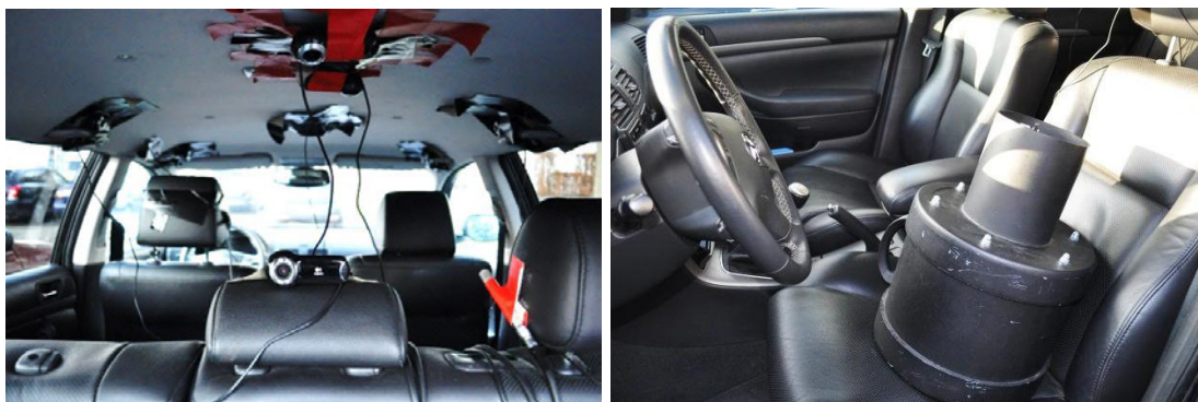
FIGURE 5.6: Distribution of cameras across the car interior (left) and monopole source (right) used in the scan-based panel contribution analysis investigation.
