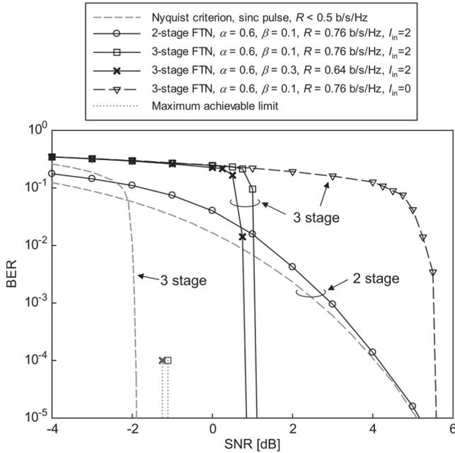
Fig. 6. Achievable BER of our FDE-aided two- and three-stage FTNS systems, employing BPSK modulation and FTNS parameter sets of  $(\alpha, \beta, \nu) = (0.6, 0.1, 10)$  and  $(0.6, 0.3, 10)$ . Moreover, we plotted the BER of the conventional Nyquist-criterion scenario. Here, we assumed the employment of the half-rate RSC(2,1,2) code, which has the polynomial generator (3,2) and a code length  $N = 2^{17}$ .
