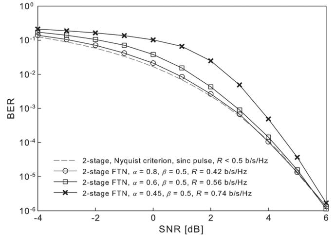
Fig. 5. Achievable BER of our FDE-aided two-stage RSC-encoded FTNS systems, employing BPSK modulation and FTNS parameters of  $(\alpha, \beta, \nu) = (0.45, 0.5, 10)$ ,  $(0.6, 0.5, 10)$ , and  $(0.8, 0.5, 10)$ . Moreover, we plotted the BER curve of the conventional Nyquist-criterion scenario as a benchmark scheme. The half-rate RSC(2,1,2) code, having the polynomial generator of (3,2) and the code length  $N = 2^{17}$ , was considered.
