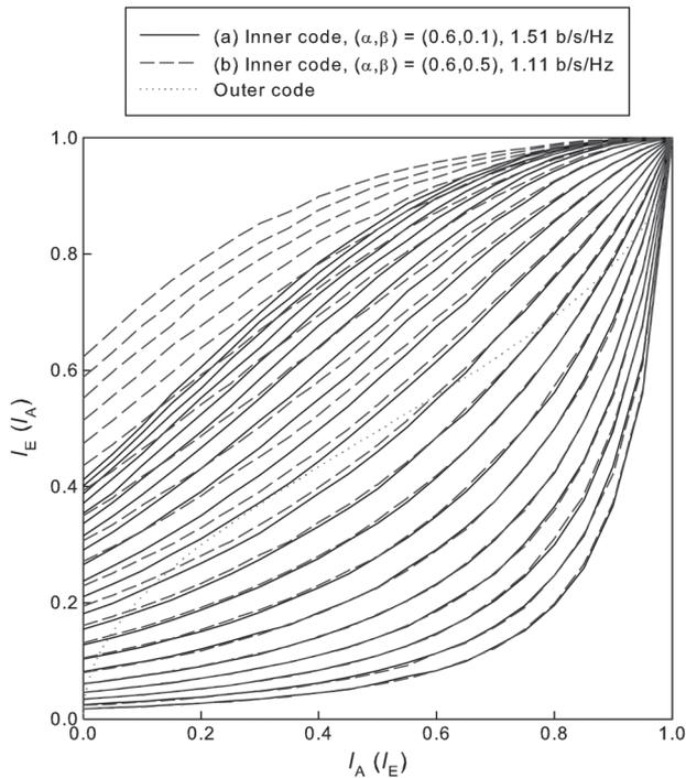
Fig. 4. EXIT charts of our three-stage concatenated FDE-aided FTNS systems, where the roll-off factor  $\beta$  was given by (a) 0.1, (b) 0.5, while maintaining the symbol's packing ratio  $\alpha = 0.6$ . The SNR of the outer code's EXIT curve was varied from  $-10$  to  $10$  dB with steps of 1 dB.
