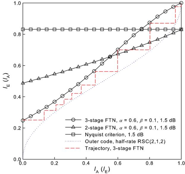
Fig. 3. EXIT charts of our FDE-aided three-stage FTNS system, employing BPSK modulation and the FTNS parameters of  $(\alpha, \beta, \nu) = (0.6, 0.5, 10)$ , where the SNR was set to 1 dB. Moreover, we plotted the inner code's EXIT curves associated with the classic Nyquist-criterion scenario, while showing the outer code's EXIT curve corresponding to the half-rate RSC(2,1,2) code, which has the generator polynomial (3,2). The code length was set to  $N = 2^{17}$ .
