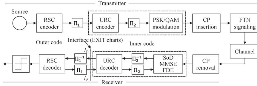
Fig. 1. Transmitter and receiver structures of our FTNS-based three-stage serially concatenated system.
