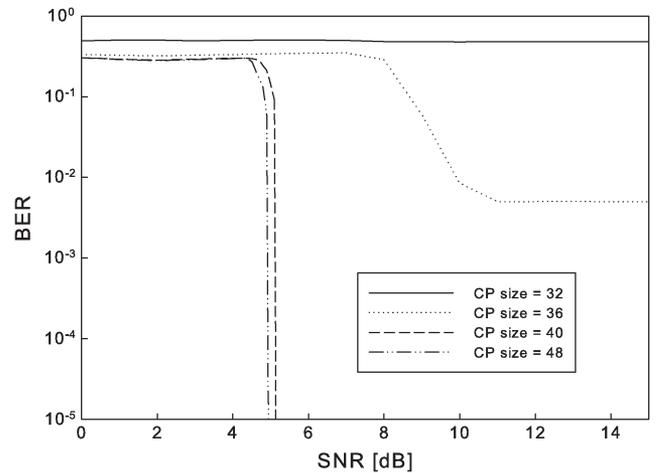
Fig. 7. Achievable BER of our FDE-aided three-stage FTNS systems, experiencing frequency-selective block Rayleigh fading, where we considered the delay spread of  $L_{DS} = 20$  taps. The BPSK modulation and the FTNS parameter set of  $(\alpha, \beta) = (0.6, 0.1)$  were employed, while varying the CP length  $2\nu$  from 32 to 48. Here, we assumed the employment of the half-rate RSC(2,1,2) code, which has the polynomial generator (3,2) and a code length  $N = 2^{17}$ .
