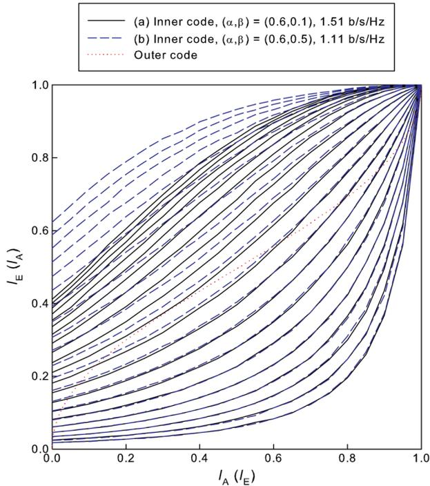
Fig. 4. EXIT charts of our three-stage concatenated FDE-aided FTNS systems, where the roll-off factor  $\beta$  was given by (a) 0.1, (b) 0.5, while maintaining the symbol's packing ratio  $\alpha = 0.6$ . The SNR of the outer code's EXIT curve was varied from  $-10$  to  $10$  dB with steps of 1 dB.
