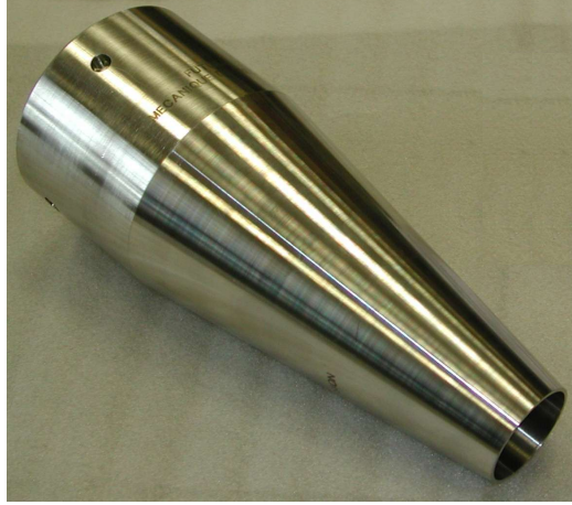
FIGURE 3.9: Photograph of the JEAN 50.0 mm diameter single stream nozzle
