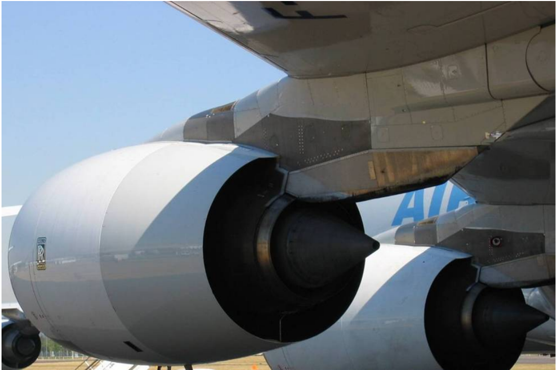
FIGURE 2.8: An under-wing-mounted modern turbofan jet engine [photo courtesy of Rolls-Royce plc.]
