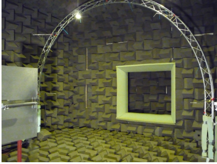
FIGURE 4.1: Photograph of the Doak Laboratory single stream jet plus horizontal flat plate far-field acoustic set-up (approximately 1/50 th model-scale)
