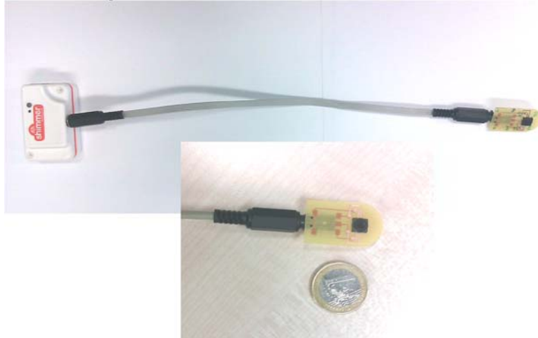
Fig. 10.12 – Prototype of the temp sweat index sensor connected to the Shimmer acceleration module.
