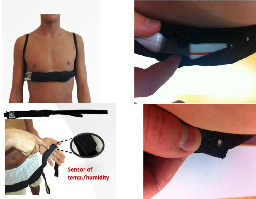
Fig.2.15 – The chest strap encapsulating the sensor modules
