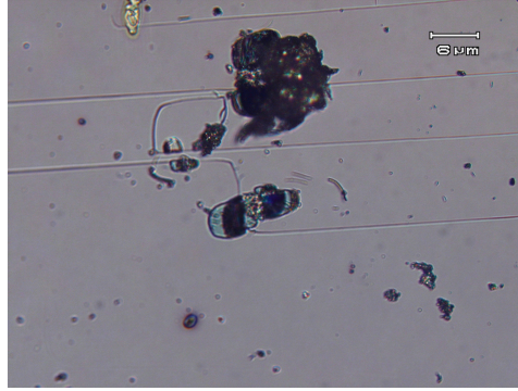
Figure 4.14: An image of the SESAM surface after it had been used in the VECSEL cavity. Damage to the surface can be seen as can furrows leading away to the left and right as a result of translating the SESAM.
