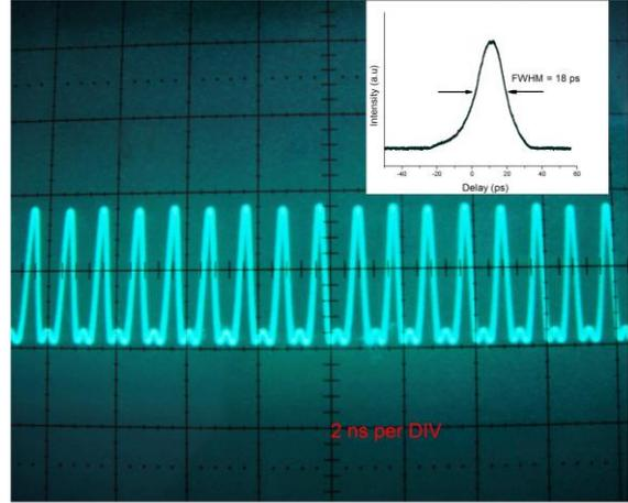
Fig. 3. Snap shot of pulse train at 16<sup>th</sup> harmonics (832.6 MHz). (Inset) Trace of intensity autocorrelator resulted in ~18 ps optical pulses.
