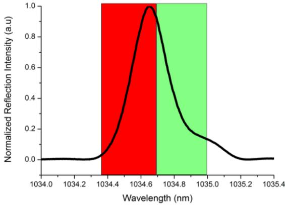
Fig. 5. Red shaded part defines the region of unstable and distorted optical pulses whilst the green shaded section represents the region for stable and clean optical pulse operation.
