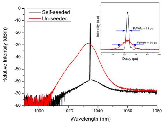
Fig. 2. Spectral profiles of the gain-switched SLD with (black line) and without (red line) FBG. (Inset) Temporal profiles for the seeded (black line) and unseeded (red line) cases.
