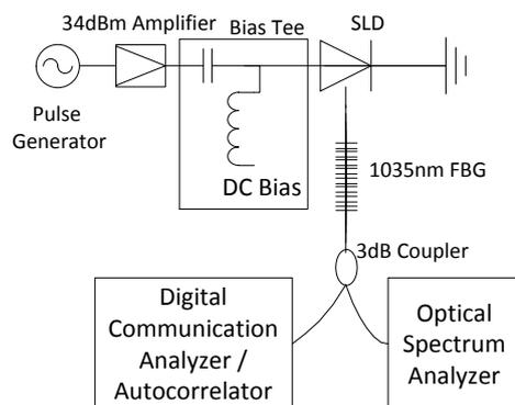
Fig. 1 Experimental setup of the picosecond pulse source.
