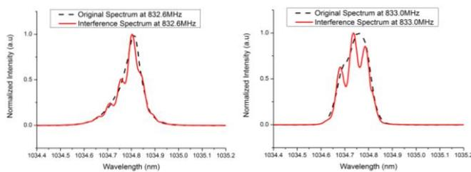
Fig. 6. Interference patterns between the 1<sup>st</sup> and the 10<sup>th</sup> optical pulses for two different operating frequencies corresponding to different operating regimes. The separation between peaks corresponds to the temporal separation between the two interfered optical pulses.
