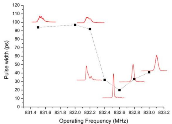
Fig. 4. Optical pulse width measured at different repetition frequencies and (Color) the corresponding optical pulse shapes
