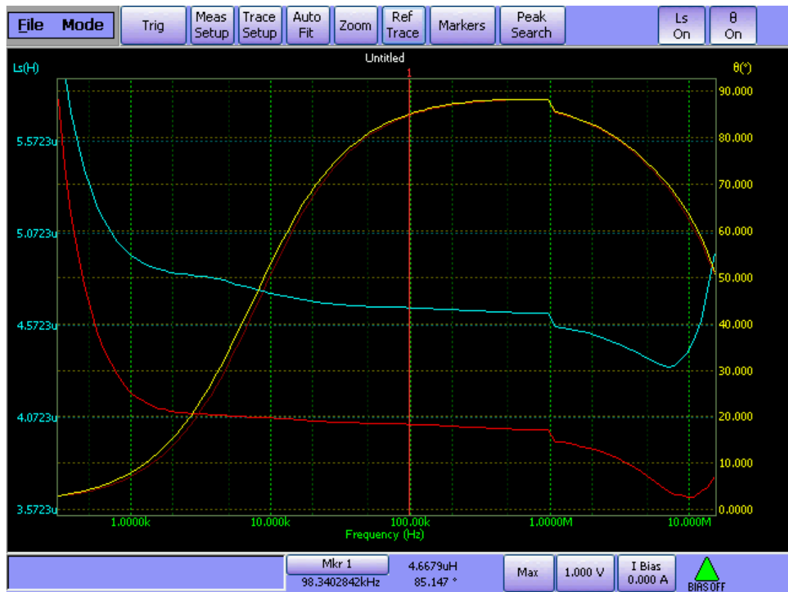
Figure A1. 4. Measured leakage inductance of the transformer primary windings; blue – primary winding 1; red – primary winding 2; yellow – phase shift
