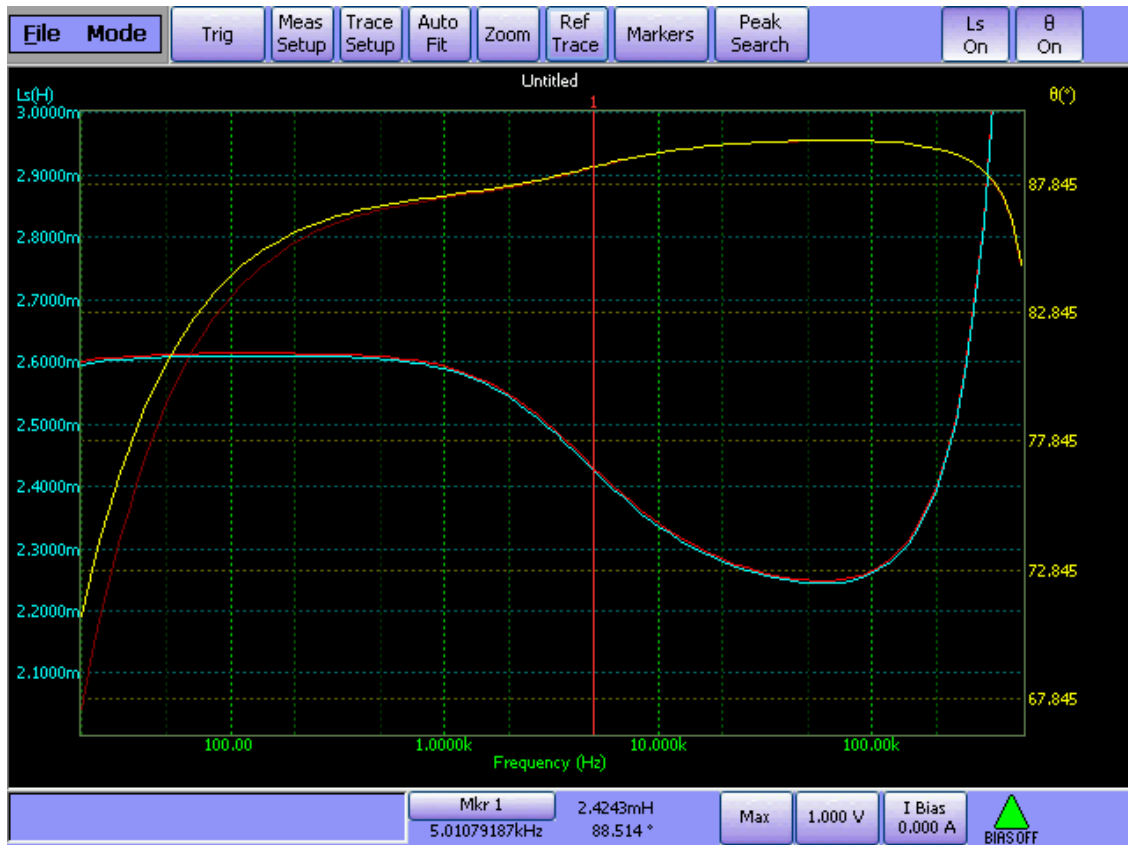
Figure A1. 2. Measured primary winding inductance; blue and red – inductance of both primary windings; yellow and brown – phase shift of the voltage across the primary windings
