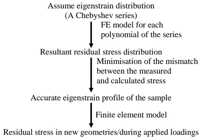
**Figure 6. Step-by-step procedure of an inverse eigenstrain analysis of the hybrid method**
