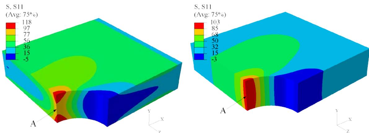
**Figure 9. a. Glass sample with residual stress under 20 MPa (X direction) tensile load (left), b. Glass sample without residual stress under 20 MPa (X direction) tensile load (right)**
