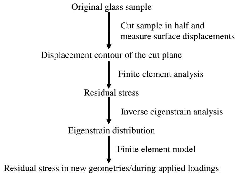
**Figure 1. Step-by-step procedure of contour/eigenstrain hybrid method**
