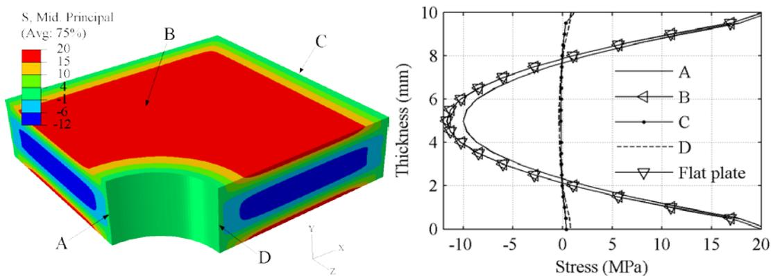
**Figure 8. a. Residual stress field (Mid. Principal) b. Stress profile in X direction (S11) at different locations in the sample**
