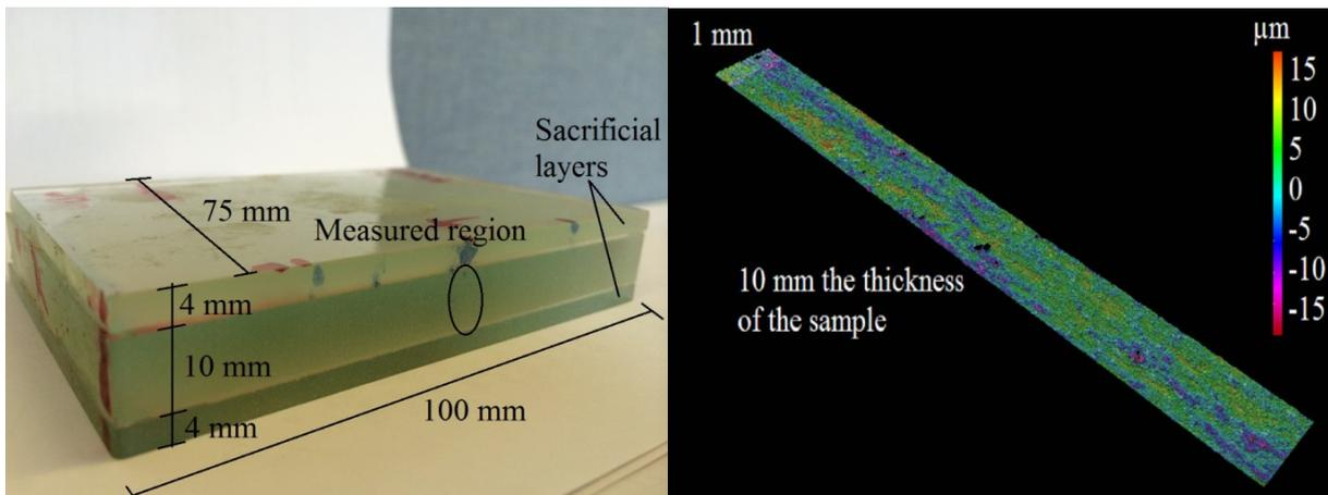
**Figure 3. a. Half of the sample after cutting (left), b. 3-D contour of the cut-plane (right)**
