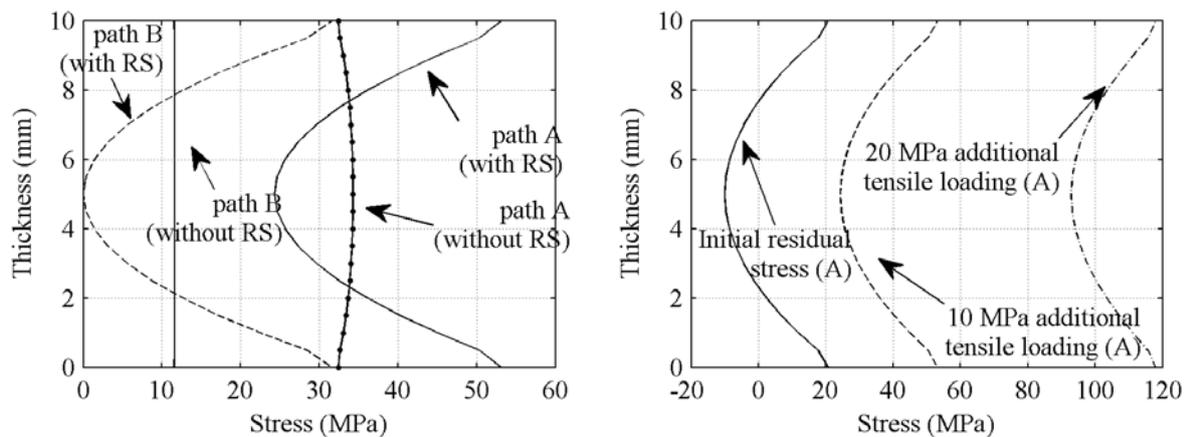
**Figure 10. a. Stress profile at 10 MPa tensile loading (left) b. Stress profile along path A for different load steps (right)**
