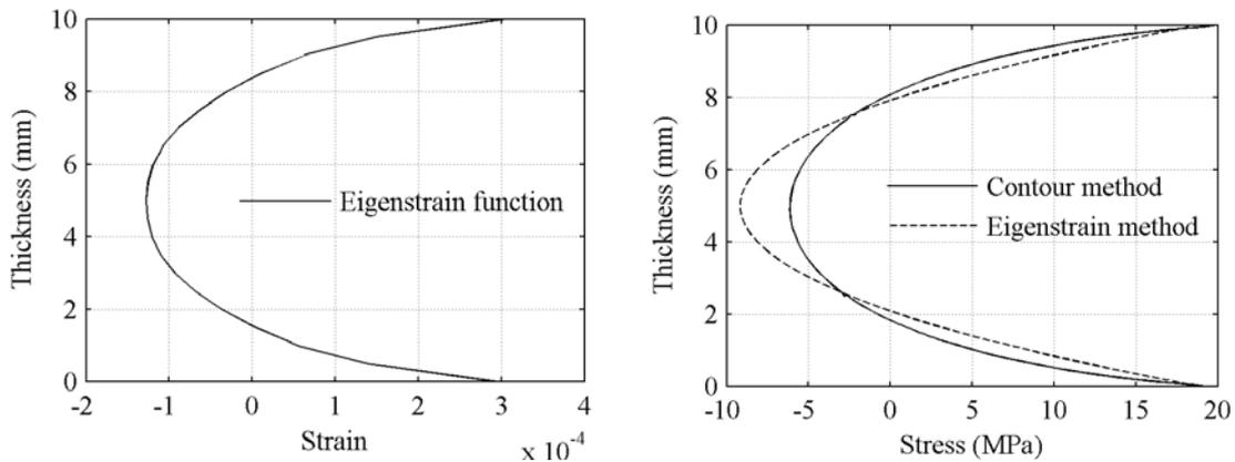
**Figure 7. a. Computed eigenstrain distribution (left) b. Comparison of stress profile (right)**
