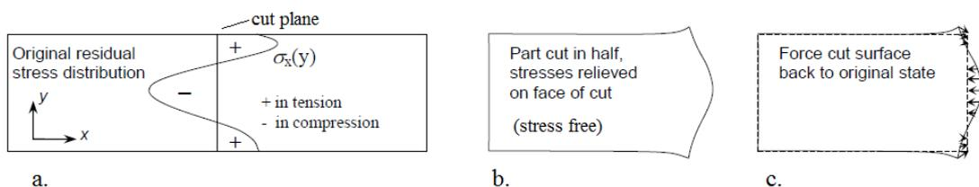
**Figure 2. Contour method principle [Prime (2001)]**
