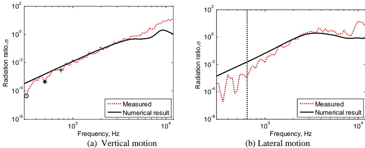
**Figure 7.** Comparison of numerical results and measurements for 1/5 scale rail in free space (the critical frequency is marked by a vertical line)
