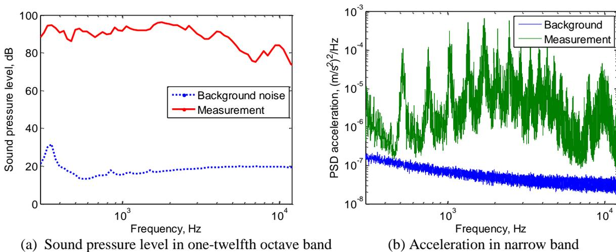
**Figure 5.** Comparison of measurement and background noise signals for rail in reverberation chamber
