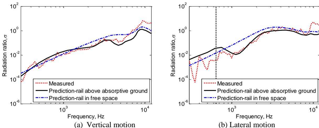
**Figure 9.** Comparison of numerical results and measurements for 1/5 scale rail 20 mm above absorptive ground
