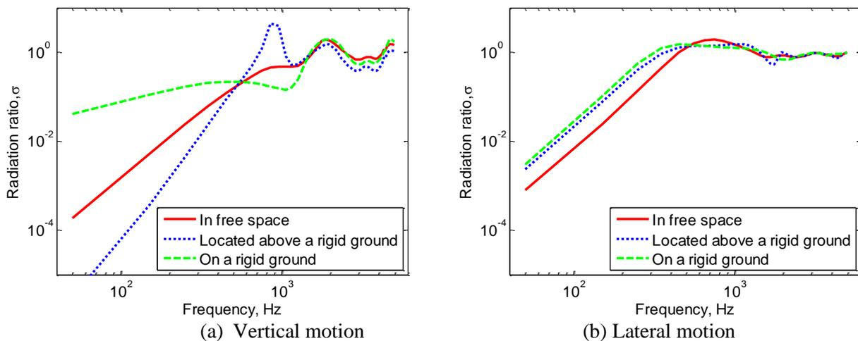
**Figure 2.** Sound radiation of the rail calculated for free space and in presence of a rigid ground
