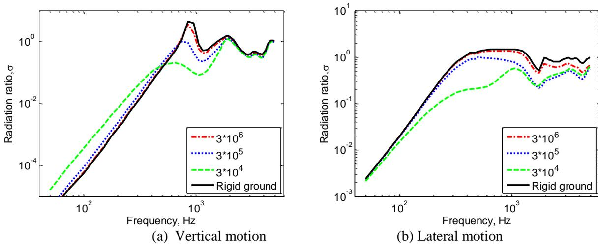
**Figure 3.** Sound radiation of the rail located 0.02 m above an absorptive ground with different values of flow resistivity
