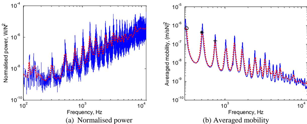
**Figure 6.** Normalised sound power and averaged mobility of rail in free space for vertical motion
