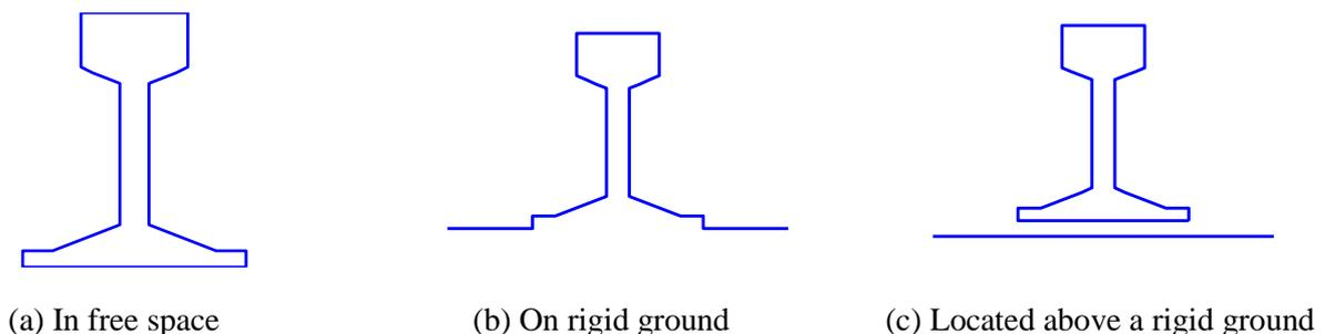
**Figure 1.** Two-dimensional Boundary Element models of a rail
