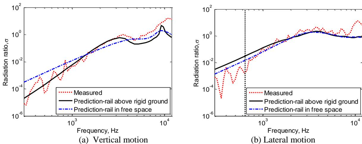
**Figure 8.** Comparison of numerical results and measurements for 1/5 scale rail 20 mm above rigid ground
