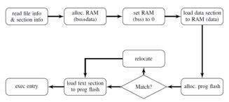
Figure 1. Dynamic linking and loading, adapted from [10]
