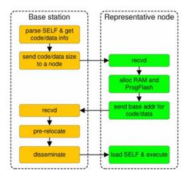
Figure 2. The pre-relocating process in SenSpire, reproduced from [10]
