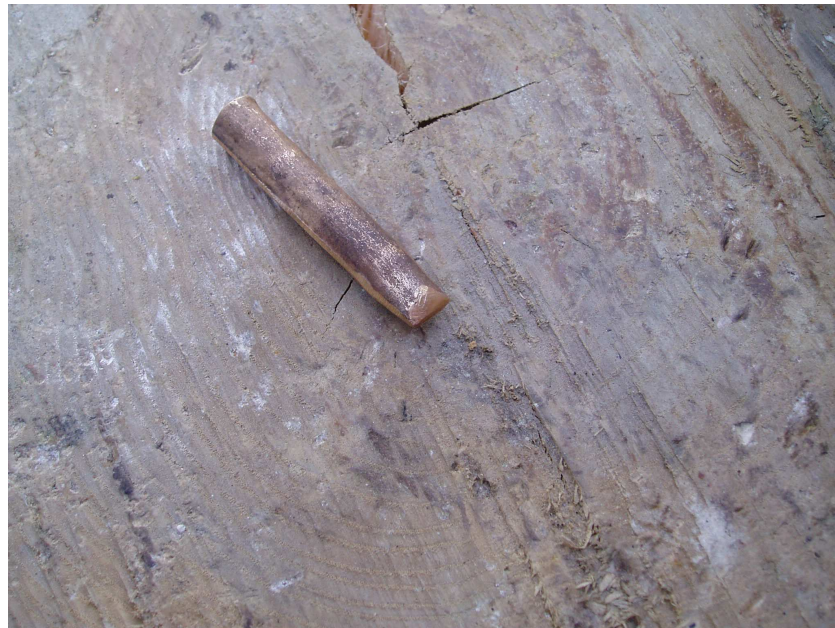
Figure 4.9 Experimental punch used to decorate test axes. Length = 6cm (Photo: Author)
