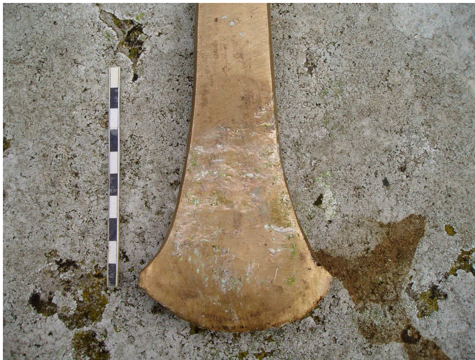
Figure 7.1 Test axe after attempts to induce fracture
