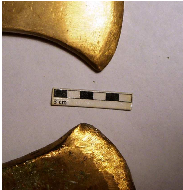
Figure 4.24 Differential blade tip wear shown on unused and used axes
