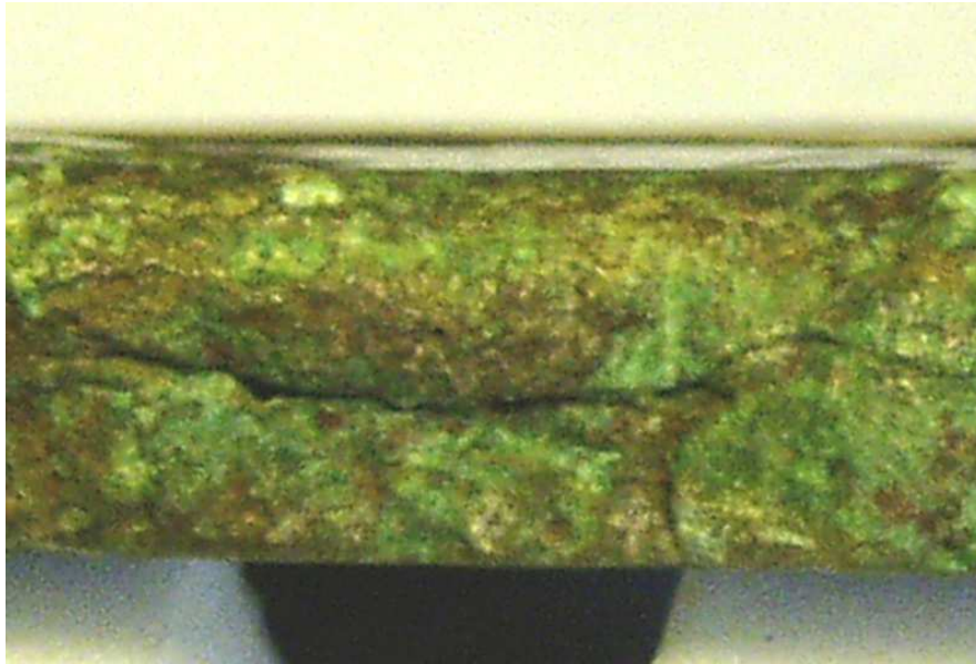
Figure 7.5: Broken axe from Auchnagarron (DA85) showing casting flaw in section
