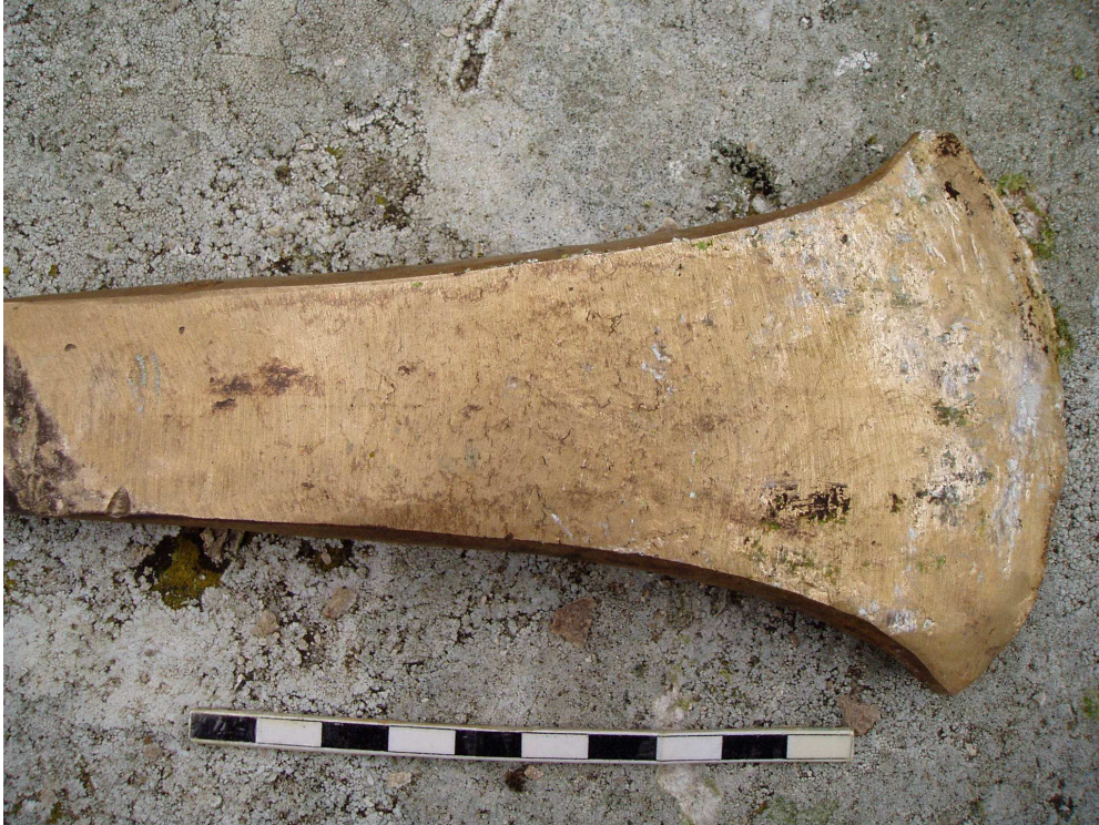
Figure 7.3 Test axe after attempts to induce fracture showing hairline cracks in surface of the axe
