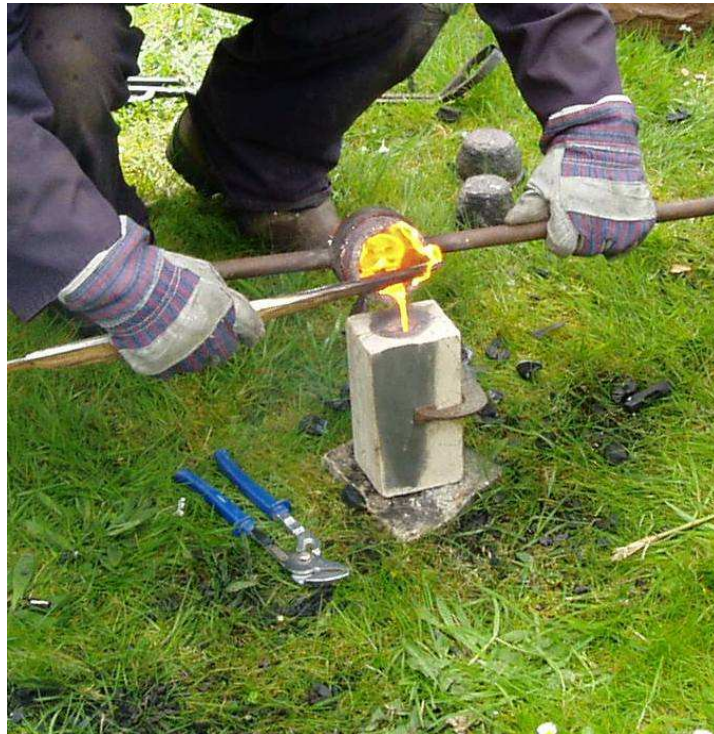
Figure 4.8 Axe 5 being cast in mould B
