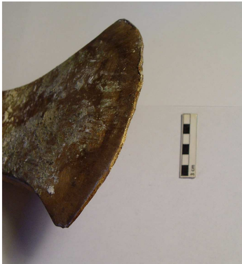
Figure 4.17 Blunt blade on an experimental axe
