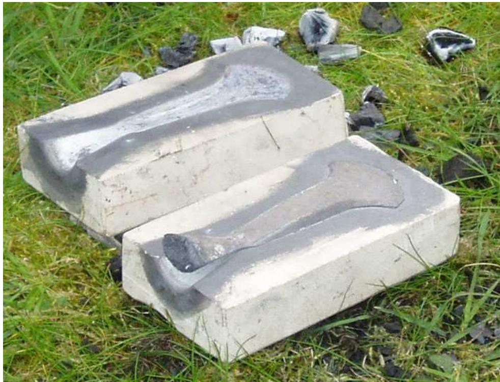
Figure 4.5 Mould B opened after casting with axe 5 in situ
