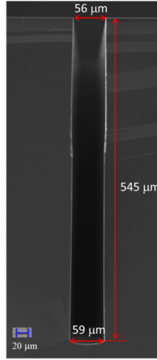
Figure 5-28: SEM image of trench after 70 minutes of backside DRIE.
