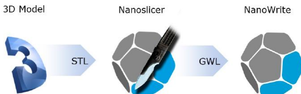
Figure 6.3: The procedure (three steps) for fabricating a 3D structure with Nanoscribe. First, the 3D structure of interest is designed by a Computer-aided design (CAD) application and exported as a Standard Tessellation Language (STL) file format. The Nanoslicer tool then reads the STL files and produces a General Writing Language (GWL) output files which are then loaded into NanoWrite to drive the direct laser writing of the structure. Picture is adopted from [139].
