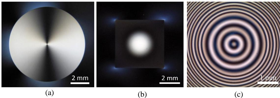
Figure 1 cross-polarized light photos of custom birefringent structures (a) radial or azimuthal polarization converter, (b) Gaussian function shaped aperture and (c) sinusoidal zone plate fabricated by femtosecond laser direct writing.
