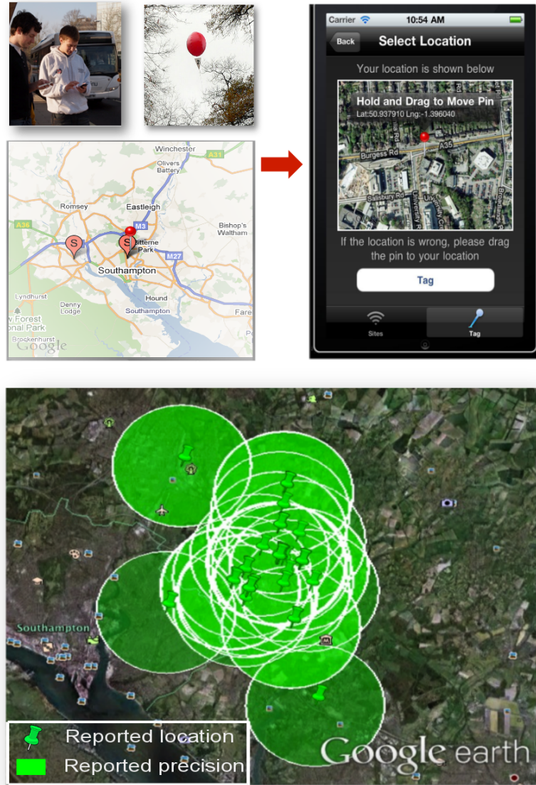
Figure 3.1: Illustration of scenario of crowdsourcing location data. The user reports GPS-based location estimates of a stationary target represented a red balloon (left most figure).
