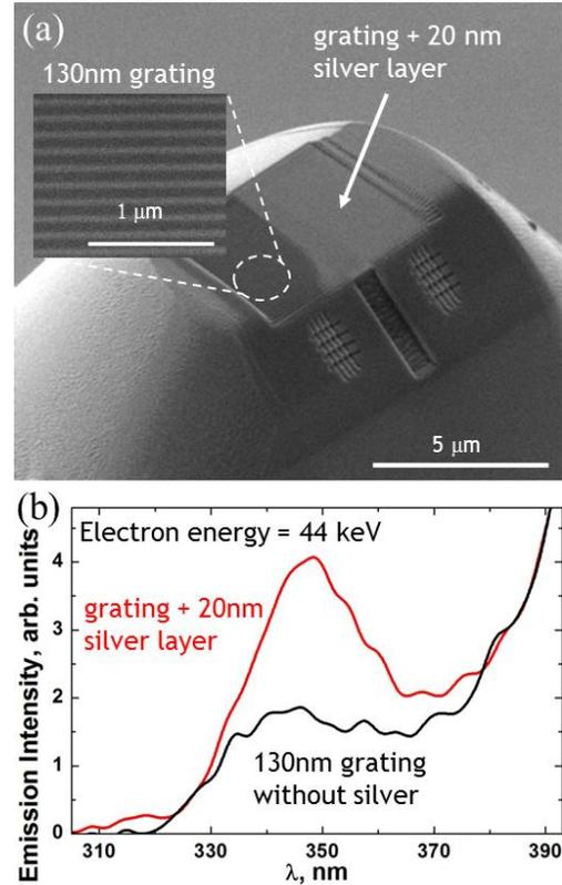
**Fig. 1:** (a) Electron microscope image of a tapered multi-mode optical fiber end face on which a planarized, 130 nm period aluminum grating has been manufactured and partially coated with a 20 nm layer of silver. (b) Electron-beam-driven light emission spectra from gratings with (red) and without (black) the silver film.
