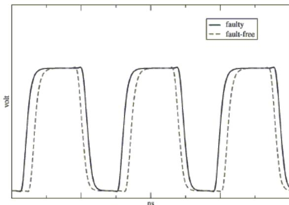
Fig. 1 Clock voltage in the fault-free case and in the case of a 50Ω bridging fault toward  $V_{dd}$ .
