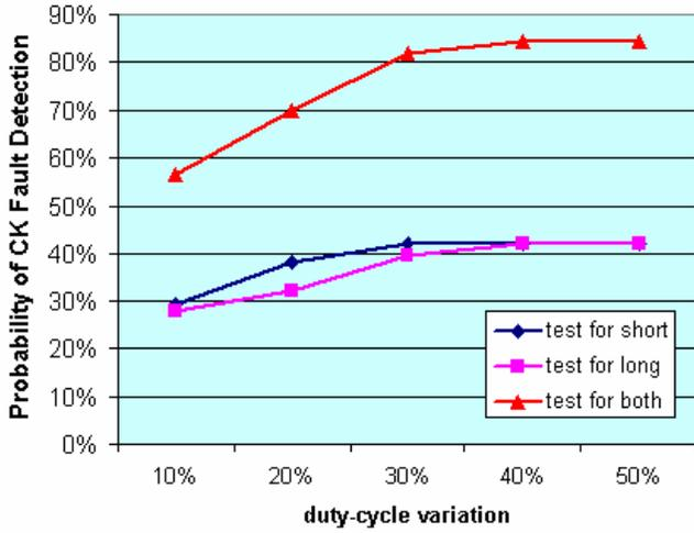
Fig. 6 CK faults detection probability by testing for min and max delay violations through functional test.
