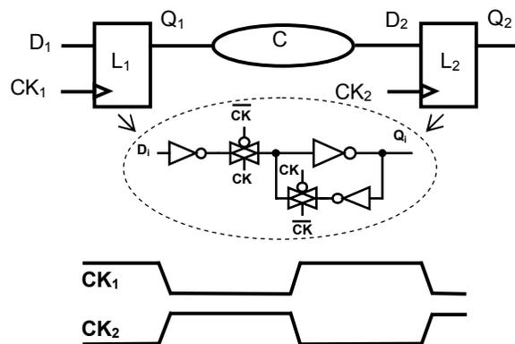
Fig. 2 Paths considered for the performed analyses.
