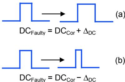
Fig. 3 Possible CK fault effect on duty cycle: clock high phase widened (a), and clock high phase shortened (b).
