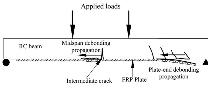
Figure 1. Debonding modes of external FRP plates
