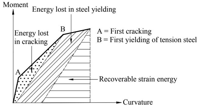
Figure 3. Energy in flexure
