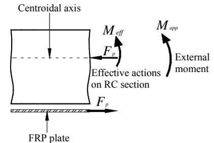
Figure 2. Actions on RC section
